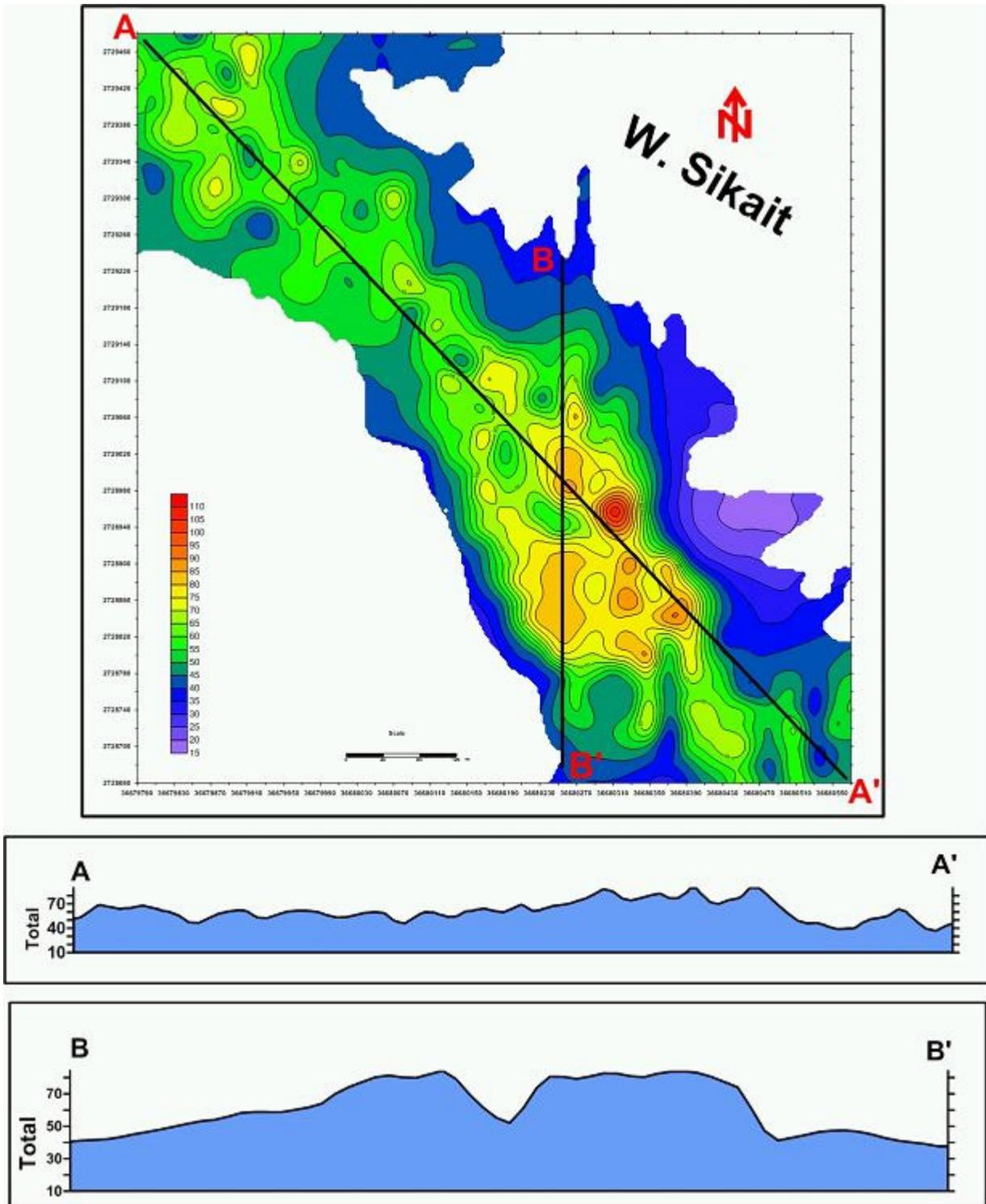
**Figure 5.** Total-count radiometric contour map for Sikait-1.
