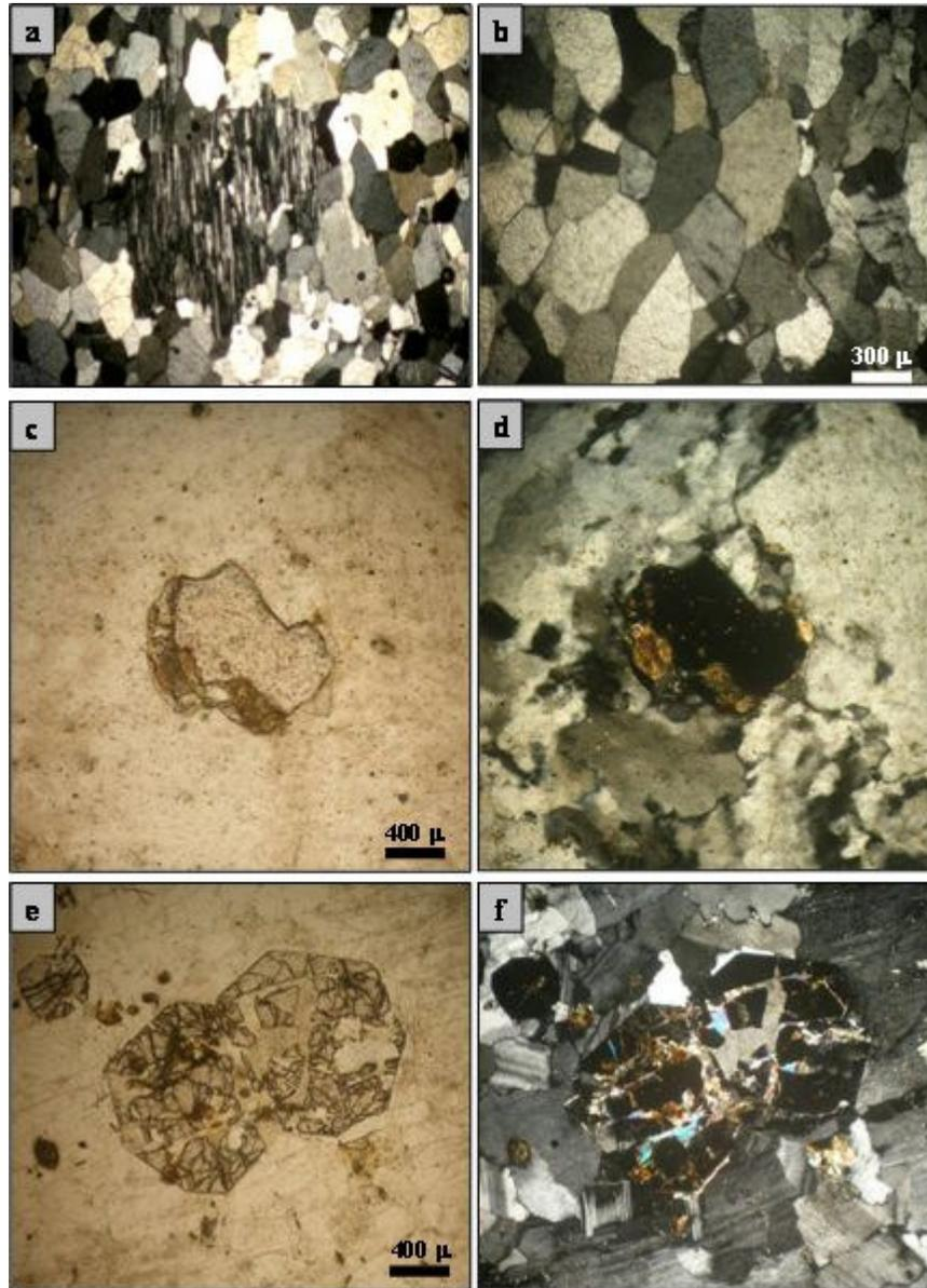
**Figure 4.** (a) View showing perthite phenocryst in greywacke, Wadi Sikait, (C.N. X20). (b) Photomicrograph showing triple junction in arkoses. Sikait, (C.N. X20). (c & d) Photomicrograph of fluorite in greywacke, P.L. (e & f) Photomicrograph of garnet in greywacke, P.L.
