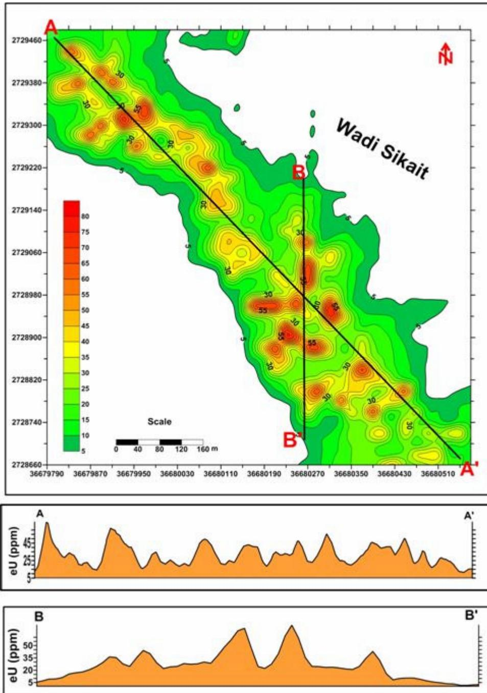
Figure 7. Equivalent uranium contour map for Sikait-1.
