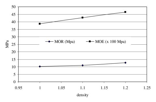
**Figure 3.** Effects of density on modulus of elasticity (MOE) and modulus of rupture (MOR) of the boards.
