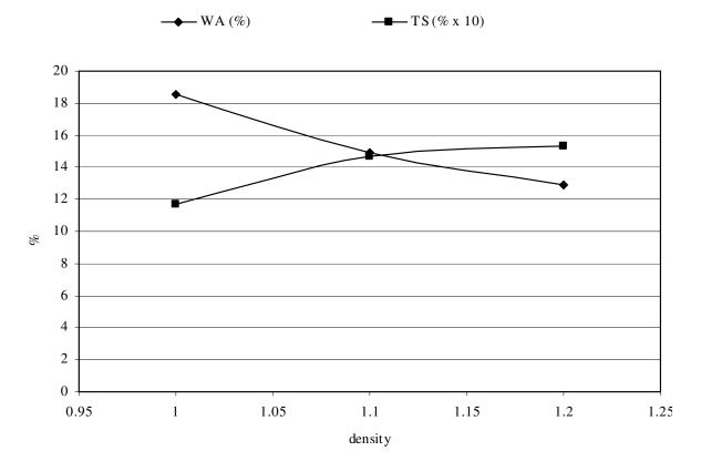
Figure 6. Effects of density on thickness swelling (TS) and water absorbtion (WA) of the boards.
