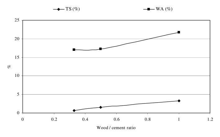
Figure 5. Effects of wood / cement ratio on thickness swelling (TS) and water absorbtion (WA) of the boards.
