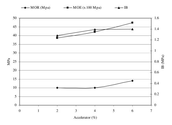
Figure 4. Effects of accelerator (%) on mechanical properties of the boards.
