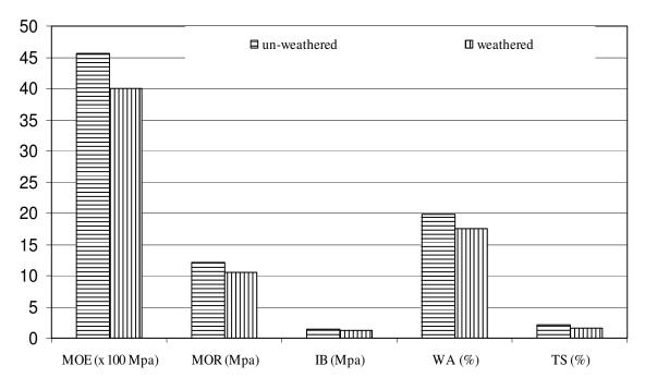
Figure 1. Effects of accelerated weathering on some physical and mechanical properties of boards.
