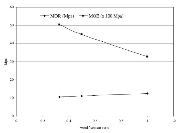
Figure 2. Effects of wood / cement ratio on modulus of elasticity (MOE) and modulus of rupture (MOR) of the boards.
