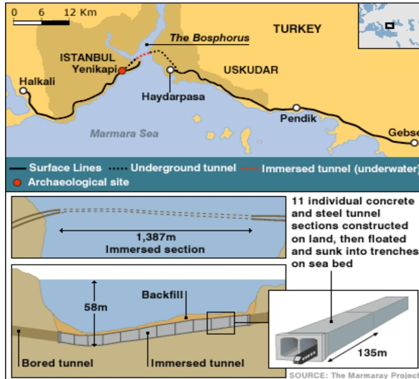
Figure 1. Bosphorus immersed tube tunnel project.
