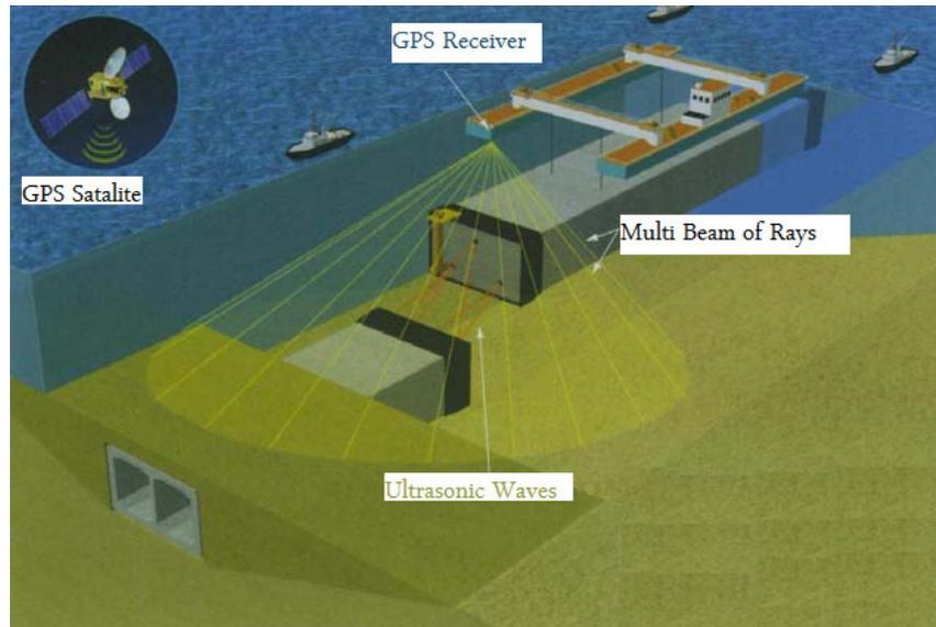
**Figure 4.** Survey works during immersion (Ünlütepe, 2005).
