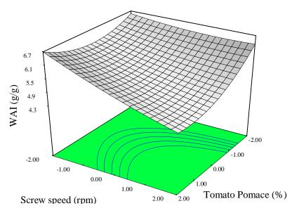
**Figure 4.** Response surface plot for water absorption index as a function of tomato pomace and screw speed.
