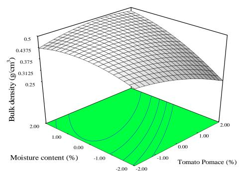
**Figure 2.** Response surface plots for the variation of bulk density as function of feed moisture and tomato pomace.
