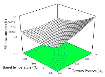
**Figure 6.** Response surface plot for maltose content as a function of tomato pomace and barrel temperature.
