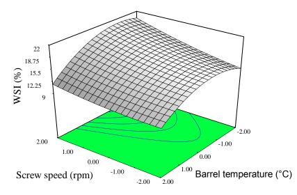
Figure 3. Response surface plot for water solubility index as a function of screw speed and temperature.
