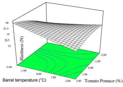
**Figure 5.** Response surface plot for hardness as a function of tomato pomace and barrel temperature.
