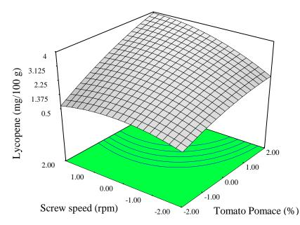
Figure 7. Response surface plot for lycopene content as a function of tomato pomace and screw speed.
