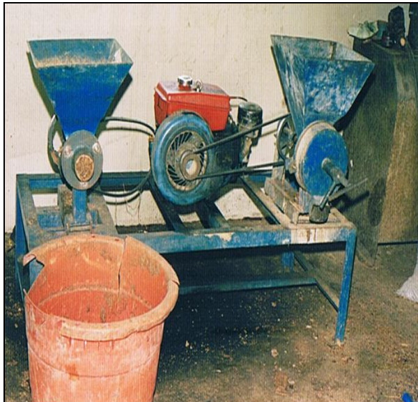
Figure 1a. Locally Fabricated diesel pelleting machine.
