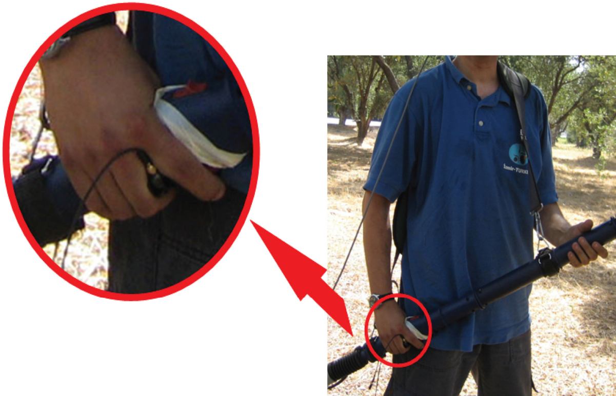
Figure 3. Position of piezoelectric accelerometer.
