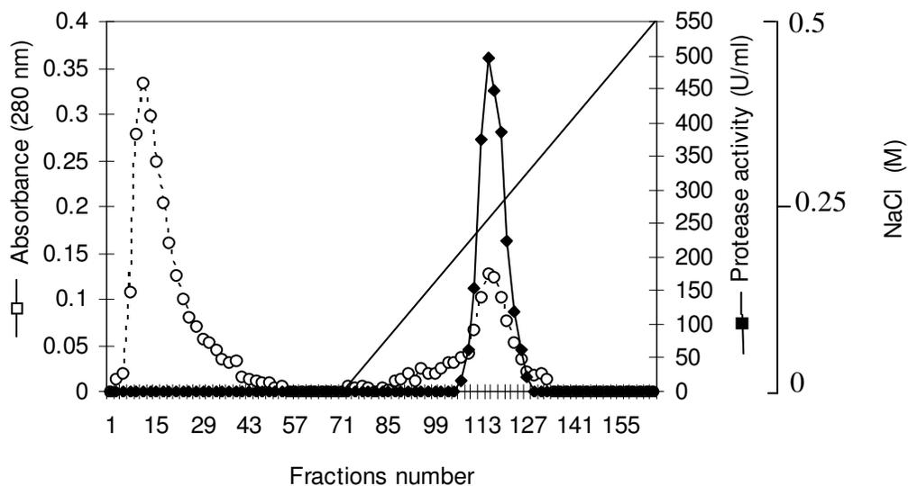
**Figure 2.** Elution profile of *A. niger* I1 protease from a CM-sephadex C-50 column. The enzyme was eluted with a linear gradient of NaCl (0-0.5 M) in glycine-HCl buffer (pH 3.0; 25 mM) at a flow rate of 120 ml/h.
