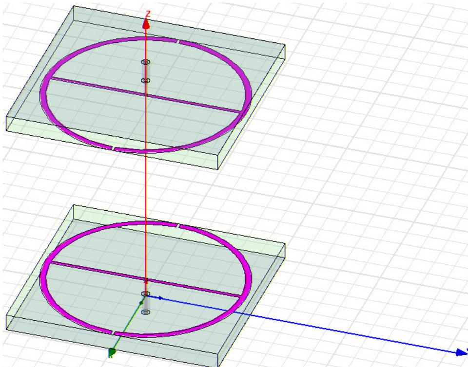
**Figure 2.** Two PSA antennas place face to face at far-field distance.
