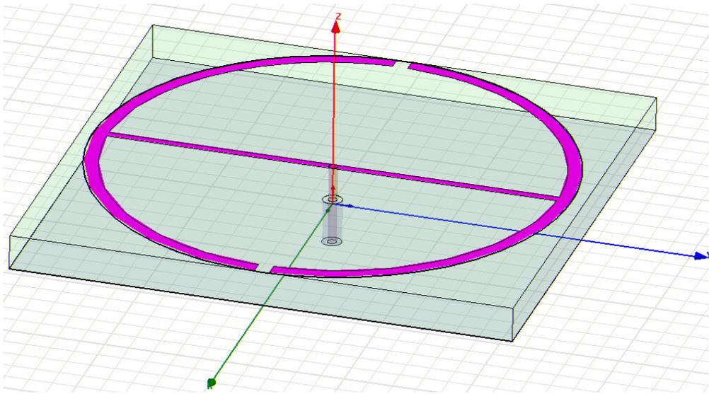
**Figure 1.** Structure of the phi shaped antenna.
