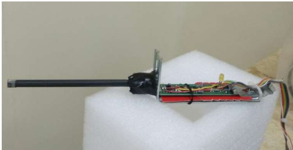
Figure 11. A completed prototype with a plastic scintillator and wave guide (both wrapped in black tape) coupled to the APD and the detection circuit.
