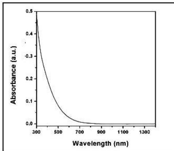
Figure 2. Optical absorption spectrum of SnS nanoparticles.
