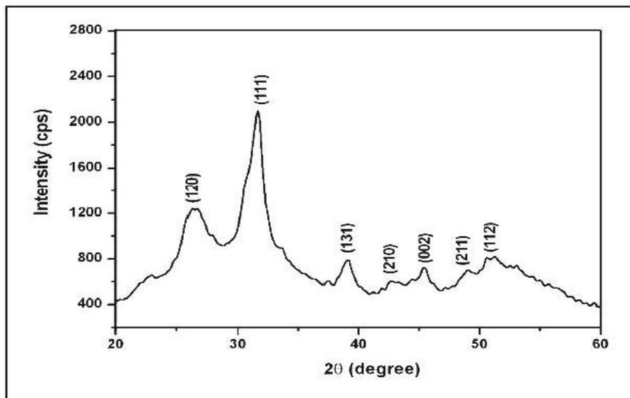
Figure 1. XRD pattern of tin sulfide nanoparticles.
