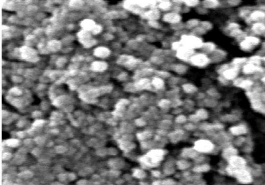
**Figure 3.** SEM image of tin sulfide nanoparticles.
