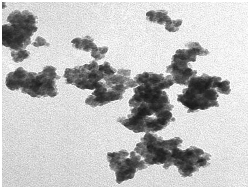
**Figure 4.** Typical TEM image of tin sulfide nanoparticles.
