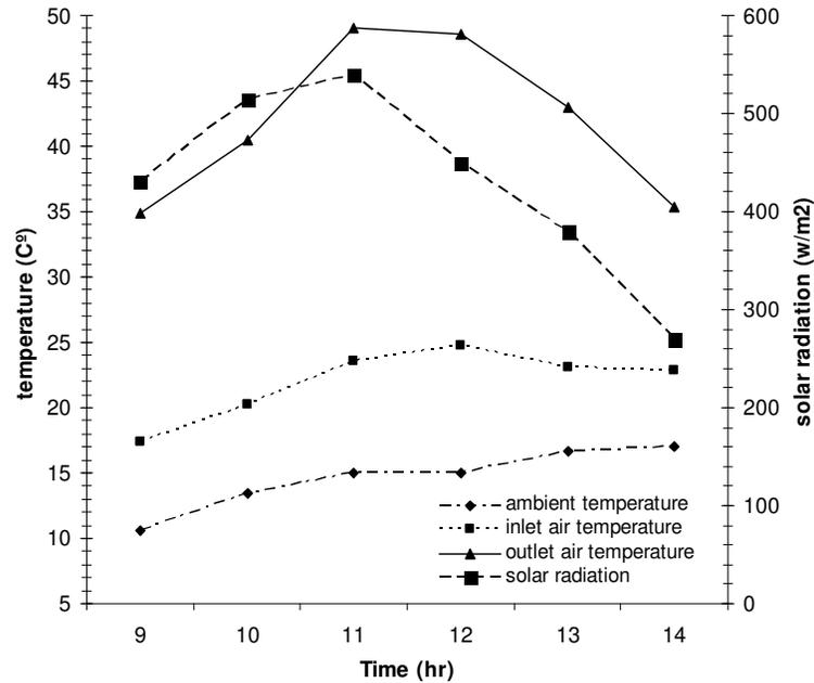
Figure 5. Time variation of air ambient temperature, air inside, outside of the collector solar and solar radiation for angle 45° (Date 22/11/2008).
