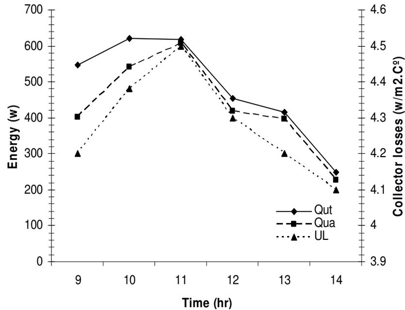
**Figure 9.** The theoretical thermal energy, the experimentally actual heats gain and the total loss factor of the collector versus the daylight hours of the inclination angle of  $60^\circ$  (Date 23/11/2008).
