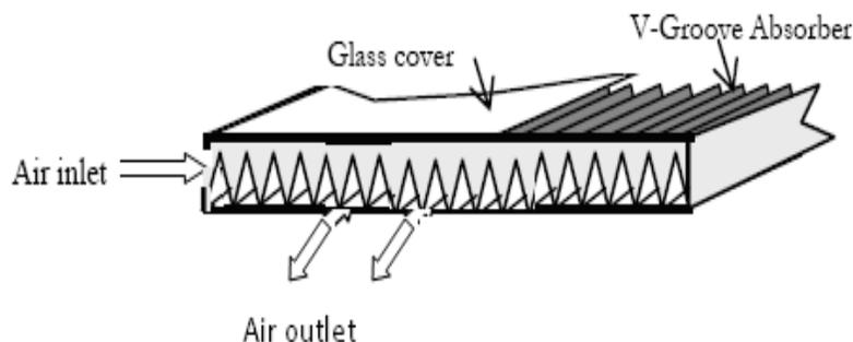
**Figure 3.** Schematic of the V-groove absorber collector.
