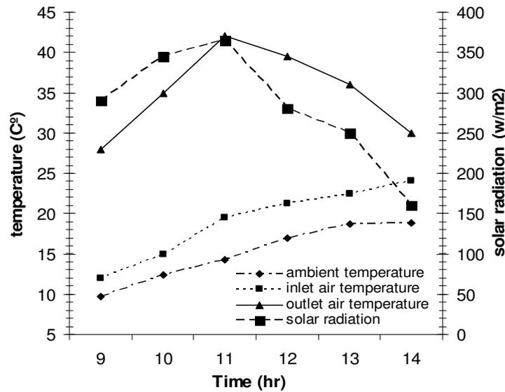
Figure 6. Air ambient temperature, air inside, outside of the collector solar and solar radiation for angle 60° (Date 23/11/2008).
