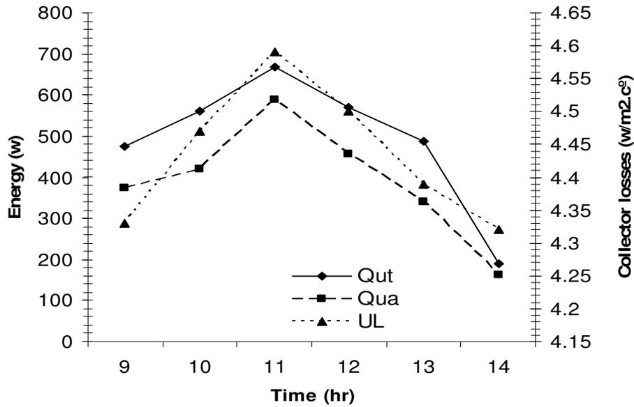
**Figure 7.** The theoretical thermal energy, the experimentally actual heat gain and the total loss factor of the collector versus the daylight hours for the inclination angle of 30° (Date 21/11/2008).
