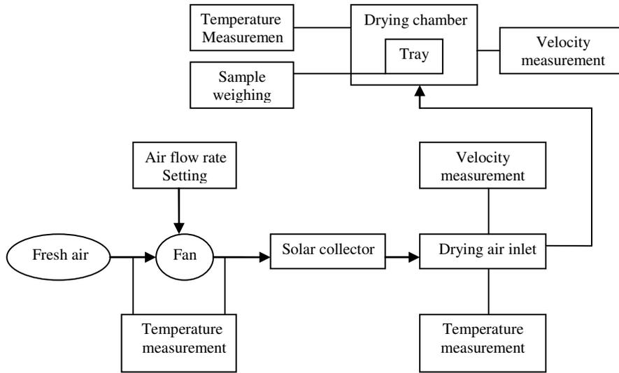
Figure 1. Flow diagram of drying process.
