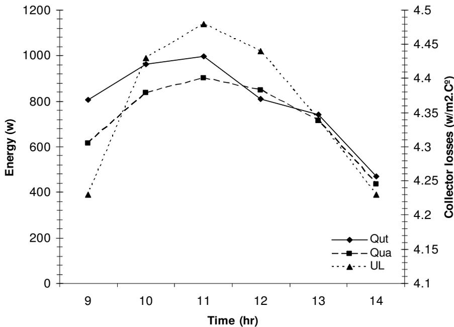
**Figure 8.** The theoretical thermal energy, the experimentally actual heats gain and the total loss factor of the collector versus the daylight hours of the inclination angle of 45° (Date 22/11/2008).
