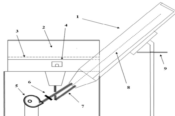
Figure 2. Section of the solar drying system: 1. Solar collector. 2. Drying chamber. 3. Drying tray. 4. Thermostat temperature. 5. Air blower. 6. Air valve. 7. Connecting pipes. 8. Absorption plates of two air passes. 9. Slide rule.
