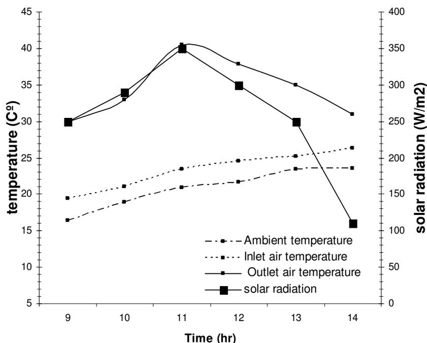
**Figure 4.** Time variation of air ambient temperature, air inside, outside of the collector and solar radiation for angle 30° (Date 21/11/2008).
