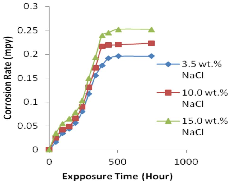
**Figure 5.** Corrosion rate of C-ring samples at different concentration of sodium chloride (NaCl) with increasing exposure time.
