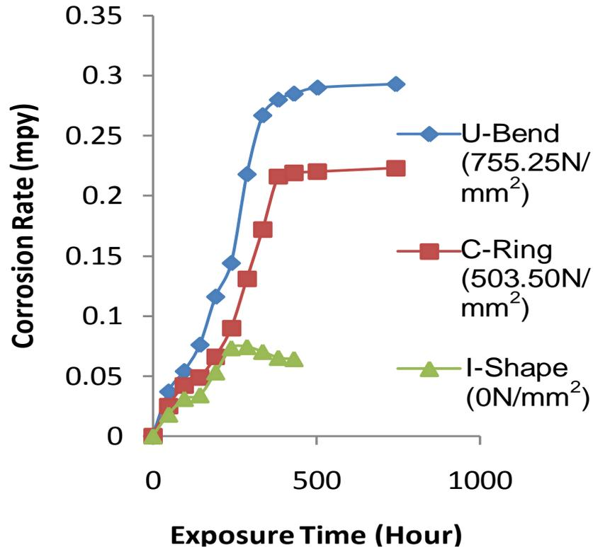
**Figure 8.** Corrosion behavior of the samples under varying stress at 10.0 wt.% NaCl with increasing exposure time.
