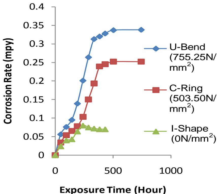
**Figure 9.** Corrosion behavior of the samples under varying stress at 15.0 wt.% NaCl with increasing exposure time.
