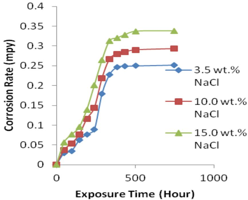
Figure 6. Corrosion rate of U-bend samples at different concentration of sodium chloride (NaCl) with increasing exposure time.
