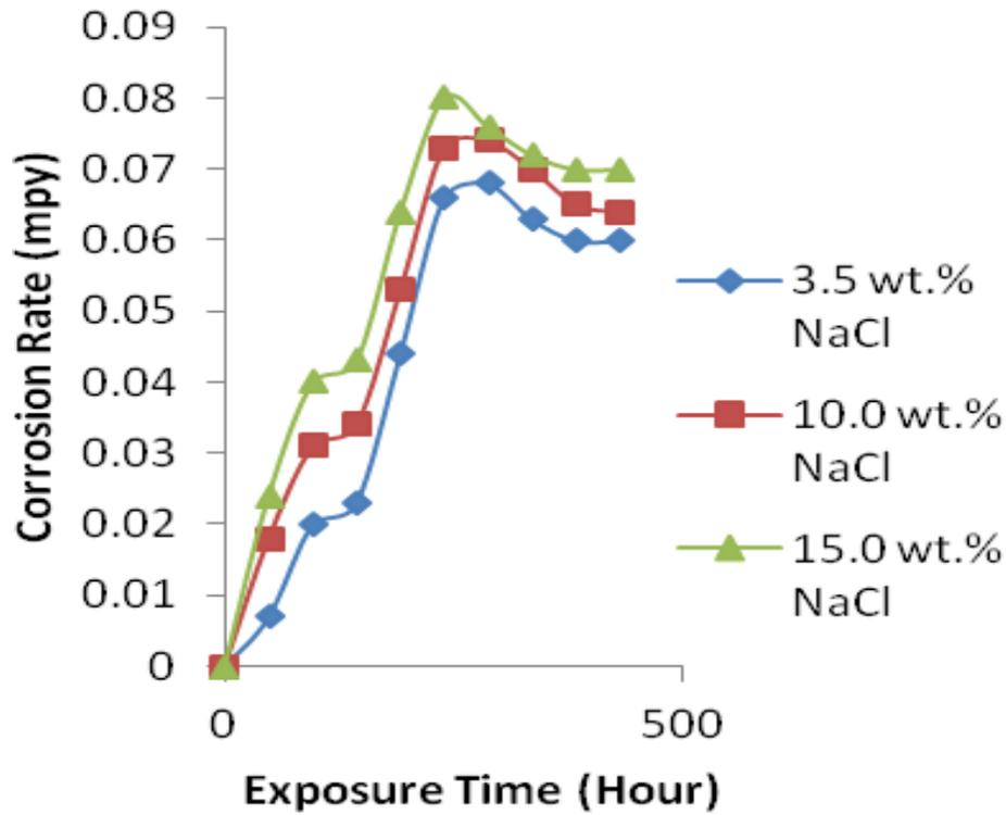
**Figure 4.** Corrosion rate of I-shape samples at different concentration of sodium chloride (NaCl) with increasing exposure time.
