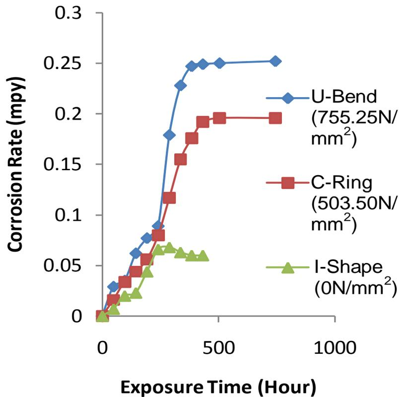
Figure 7. Corrosion behavior of the samples under varying tensile stress at 3.5 wt.% NaCl with increasing exposure time.
