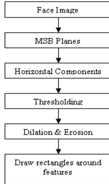
Figure 9. Sequential block diagram of the proposed method.
