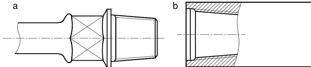
**Figure 2.** A schematic of tapered thread: (a) Joint, and (b) coupling.
