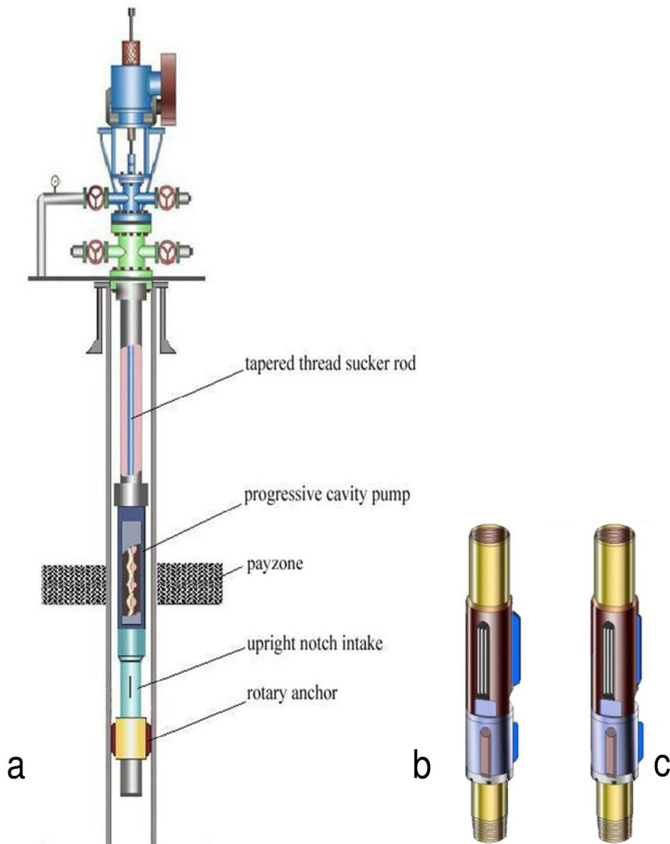
**Figure 4.** (a) Schematic of the modified PCP system together with pump intake configuration: (b) Rotary anchor in operational state, and (c) Rotary anchor in idle state.
