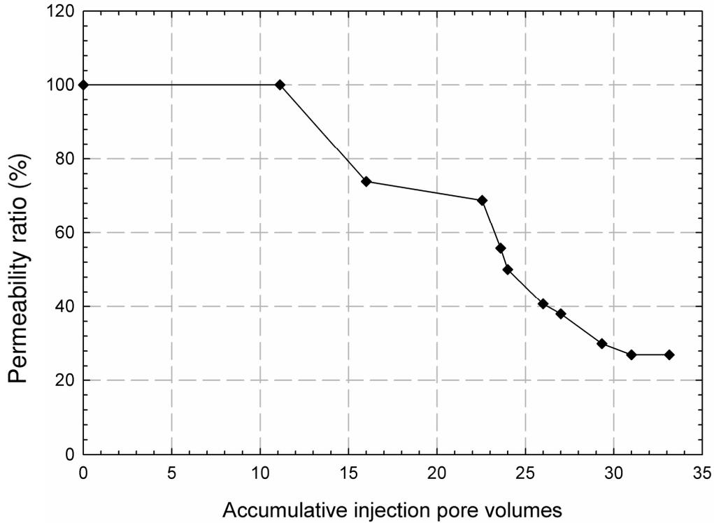
**Figure 1.** Ratio of permeability due to water injection to its original permeability as a function of accumulative pore volume of the injected water during a conventional water sensitivity test.
