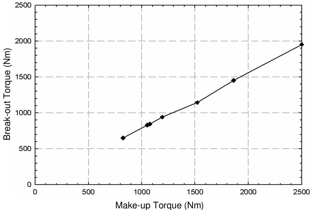
Figure 3. Measured make-up and break-out torques.
