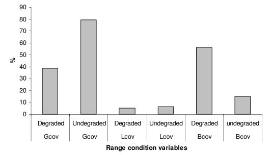
**Figure 2.** Mean grass cover (%), litter cover (%) and bare soil cover (%) estimated in the randomly selected plots using 1  $m^2$  metal frame quadrats on degraded and undegraded plots in the Umfolozi catchment (Gcov = grass cover, Lcov = litter cover, Bcov = bare soil cover).
