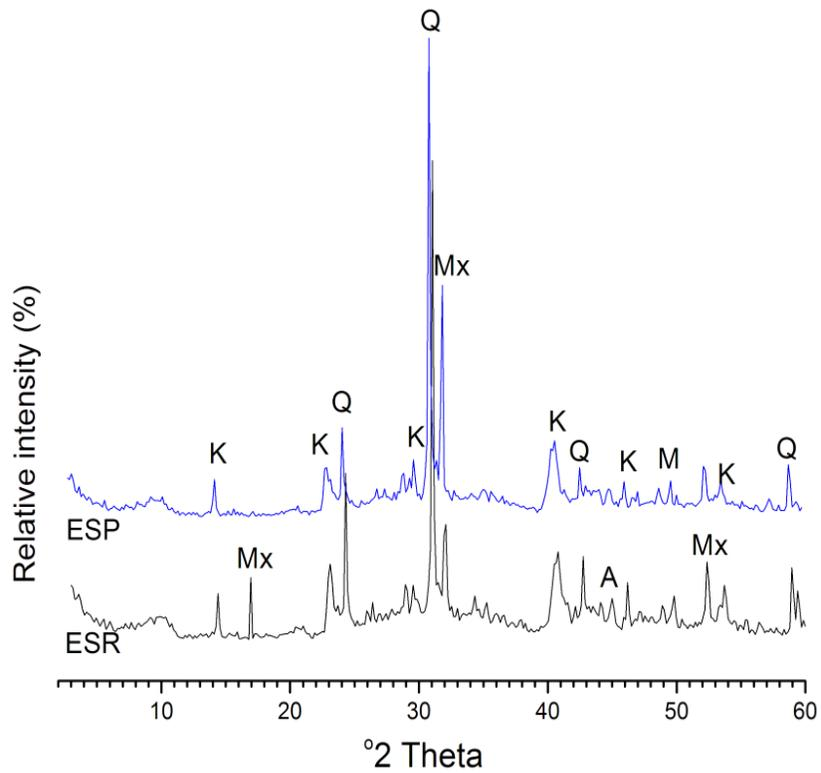
**Figure 3.** X-ray diffractogram of representative bulk kaolin samples (K: kaolinite, M: muscovite, Q: quartz, A: anatase, Mx: microcline).
