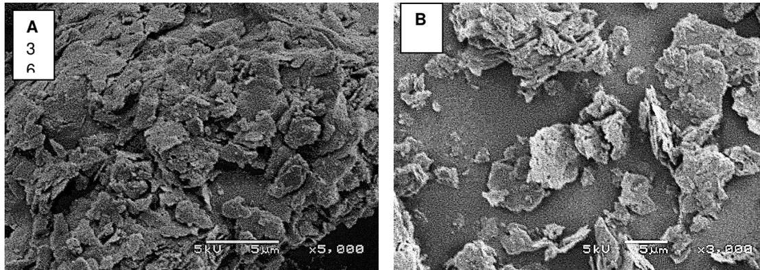
**Figure 5.** SEM photomicrograph of representative samples from Ediki kaolin occurrence; (a) laths, irregular platelets and flakes with swirl texture and rounded edges; (b) loose stacks and flakes.
