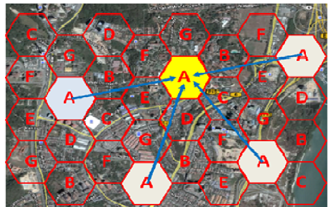
Figure 9. The new proposed topology (N = 7) for the same sample area as shown in Figure (2). There will be the same step and connection for cell groups B, C, D, E, F, and G because N = 7; the yellow-colored cell is the CBS for this cell group.
