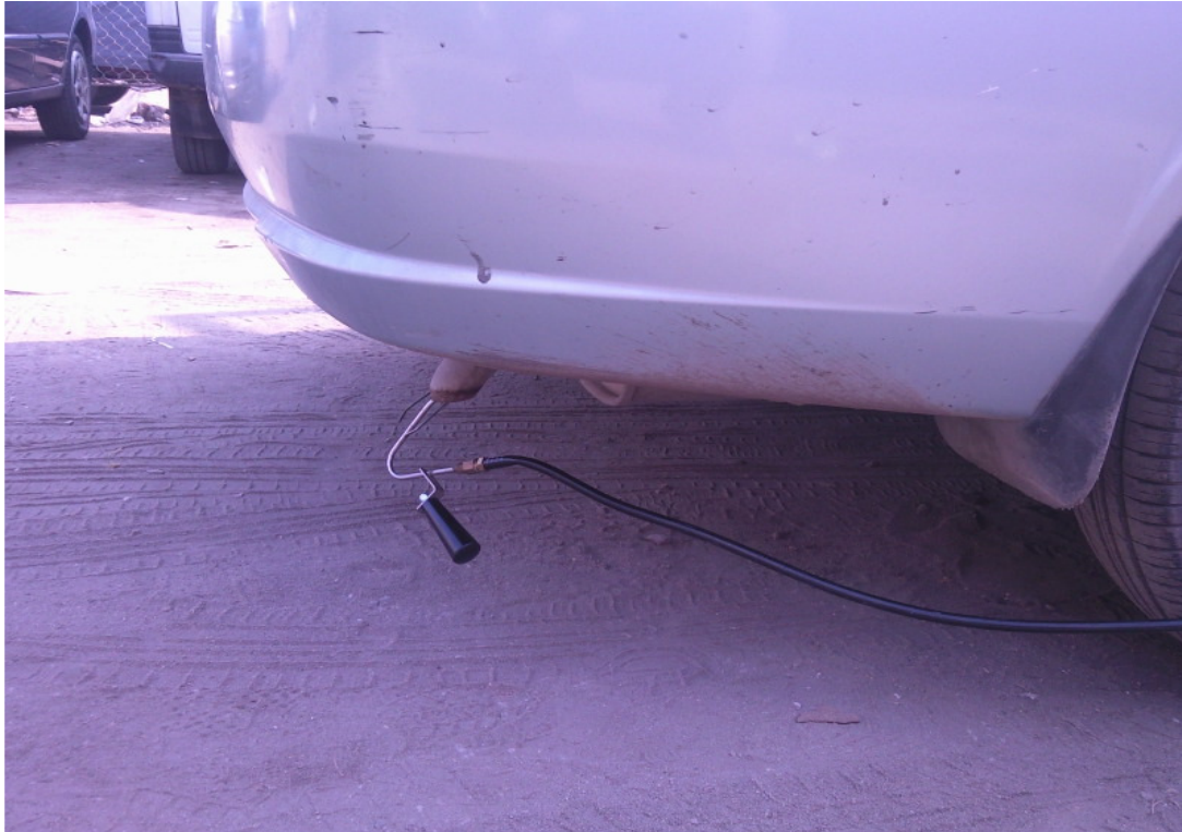
Figure 6. The probe inside the exhaust tailpipe.
