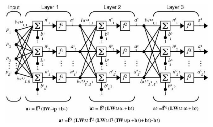
Figure 3. Three layer feed forward artificial neural network.
