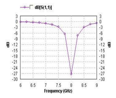
Figure 2. The return loss  $(S_{11})$  in dB verses resonating frequency of microsrip antenna.
