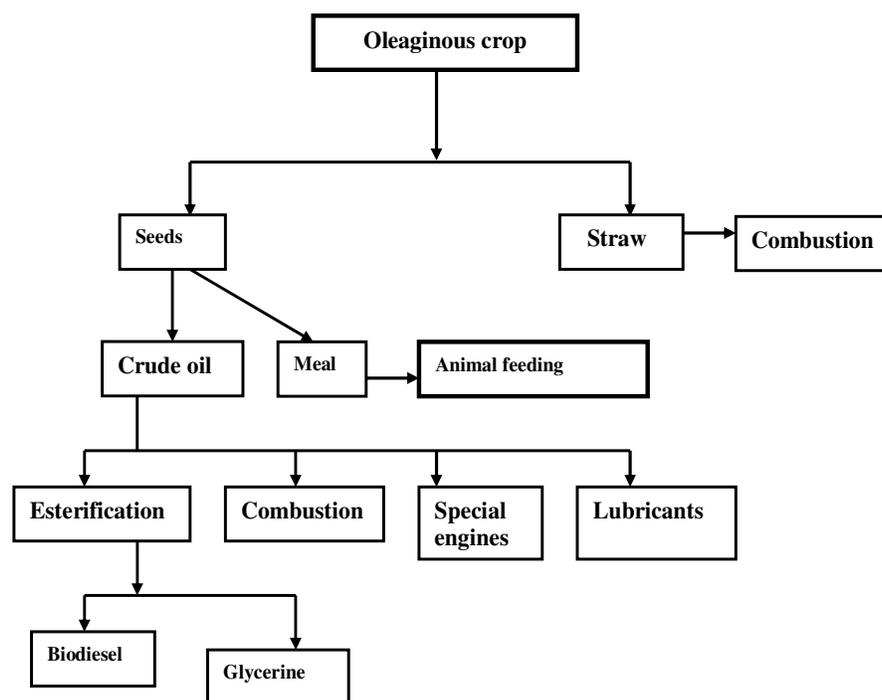
**Figure 7.** Flow chart of biodiesel production.
