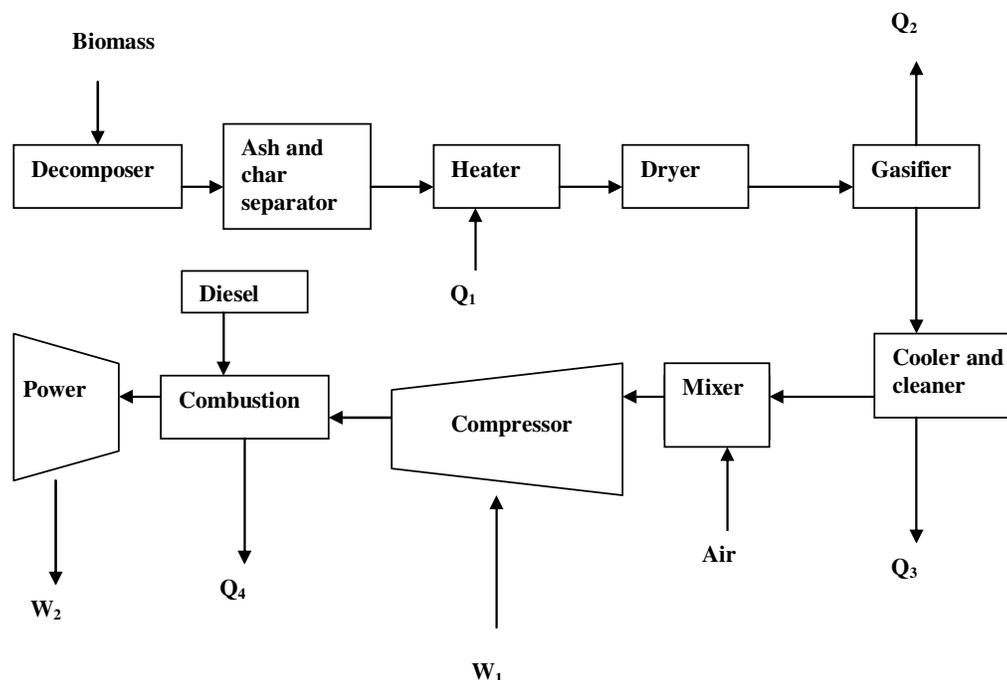
**Figure 5.** Advanced biomass power with diesel engine.
