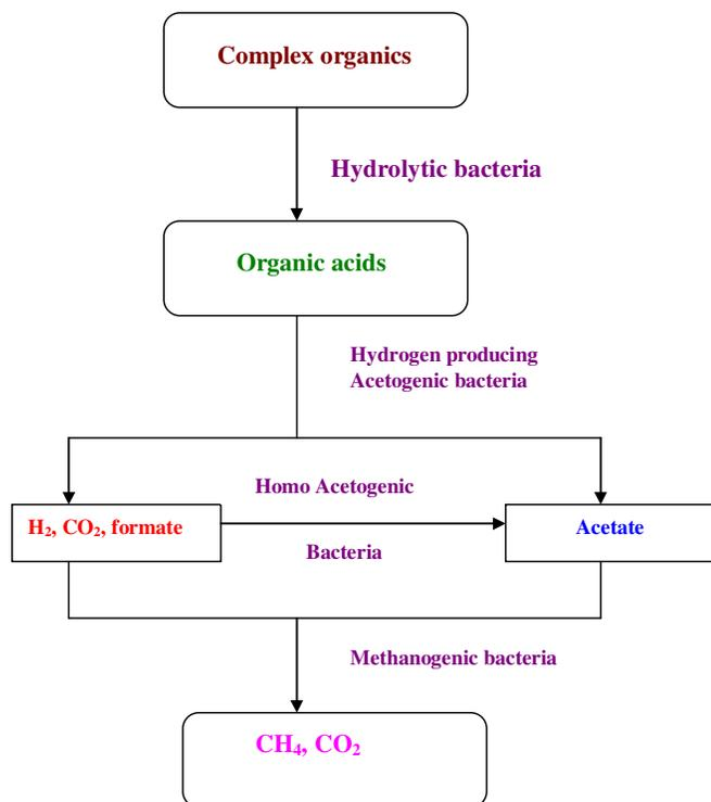
**Figure 2.** Biogas production process (Omer, 2003).
