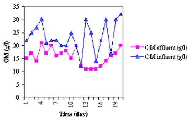
**Figure 3.** Organic matters before and after treatment in digester.
