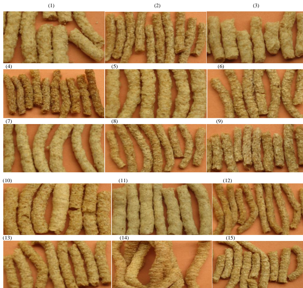
Figure 1 (Plate 1 to 15): (1) 10% Cowpea, 20% moisture, 150rpm; (2) 10% Cowpea,30%moisture, 150rpm; (3) 10% Cowpea, 20% moisture, 250 rpm; (4) 10% Cowpea, 30% moisture, 250 rpm; (5) 30% Cowpea, 20% moisture, 150 rpm; (6) 30% Cowpea, 30%moisture, 150 rpm; (7)30% Cowpea, 20% moisture, 250rpm.;(8) 30% Cowpea, 30% moisture, 250 rpm; (9) 3.2% Cowpea, 25% moisture, 200 rpm; (10) 36.8% Cowpea, 25% moisture, 200 rpm; (11) 20% Cowpea, 16.6% moisture, 200 rpm; (12)20% Cowpea, 33.4% moisture, 200rpm; (13)20% Cowpea, 25% moisture, 116 rpm; (14) 20% Cowpea, 25%, moisture, 284 rpm; (15) 20% Cowpea, 25% moisture, 200 rpm.
