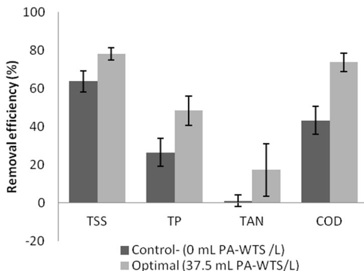
**Figure 3.** Average percentage removals ± SD of COD, TSS, TAN and TP for the control and the optimal dose at 5 min mixing time and settlement of 30 min.
