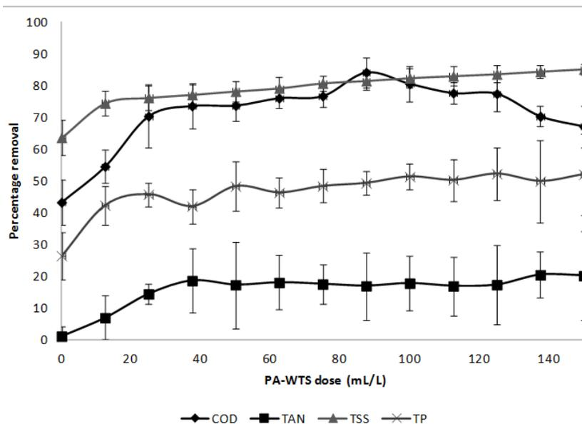
**Figure 2.** Effect of different doses of the PA-WTS on COD, TSS, TAN and TP removal efficiency from wastewater.
