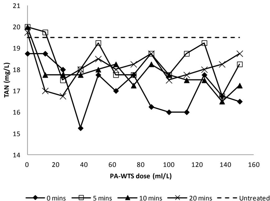
**Figure 1A.** TAN values for wastewater supernatant after adding different PA-WTS doses at different mixing times and settlement time of 30 min.
