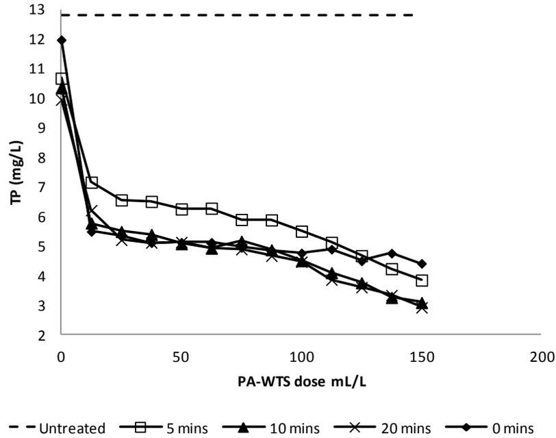
**Figure 1C.** TP values for wastewater supernatant after adding different PA-WTS doses at different mixing times and settlement time of 30 min.
