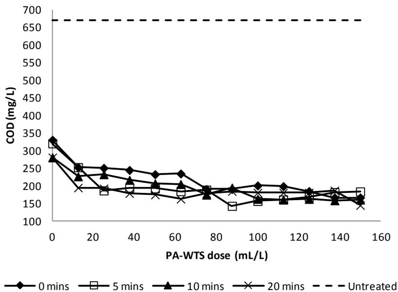
**Figure 1B.** COD values for wastewater supernatant after adding different PA-WTS doses at different mixing times and settlement time of 30 min.
