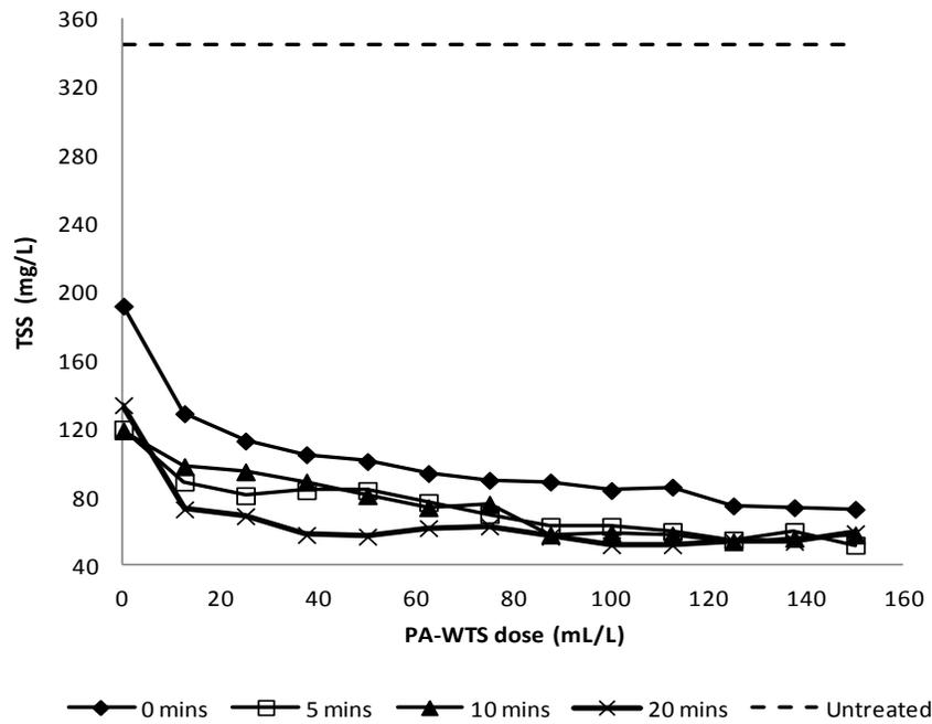
**Figure 1D.** TSS values for wastewater supernatant after adding different PA-WTS doses at different mixing times and settlement time of 30 min.
