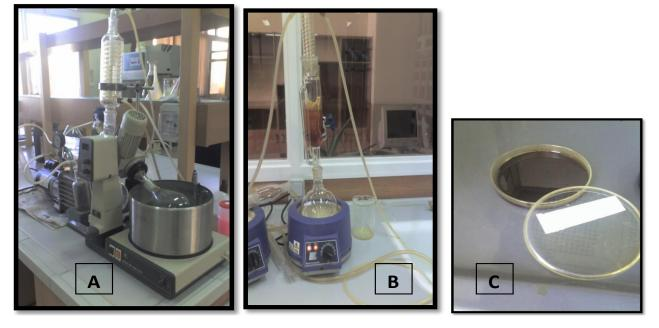
Figure 1. A: Soxhelet apparatus; B: Rotaevaporatory system; C: Plants extract after fully evaporation which is tar shape.
