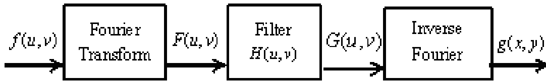
Figure 1. The principle and process of the frequency domain method.
