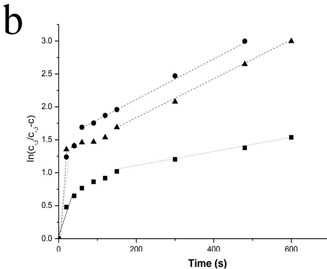
**Figure 2.** Kinetics of F extraction at 70°C. a: Changes in F concentration with extraction time; b: Functional relationship of  $\ln[c_{t,3}/(c_{\infty}-c)]$  with time. Particle mean size: ▲, 0.113 mm; ●, 0.160 mm; ■, 0.380 mm.
