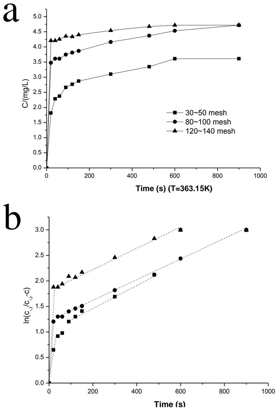
**Figure 3.** Kinetics of F extraction at 90°C. (a) Changes in F concentration with extraction time; (b) Functional relationship of  $\ln(c_{\infty}/(c_{\infty}-c))$  with time. Particle mean size: ▲, 0.113 mm; ●, 0.160 mm; ■, 0.380 mm.
