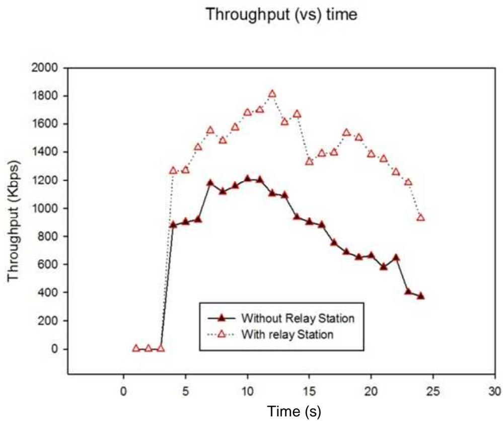
Figure 15. Throughput with and without relay station.
