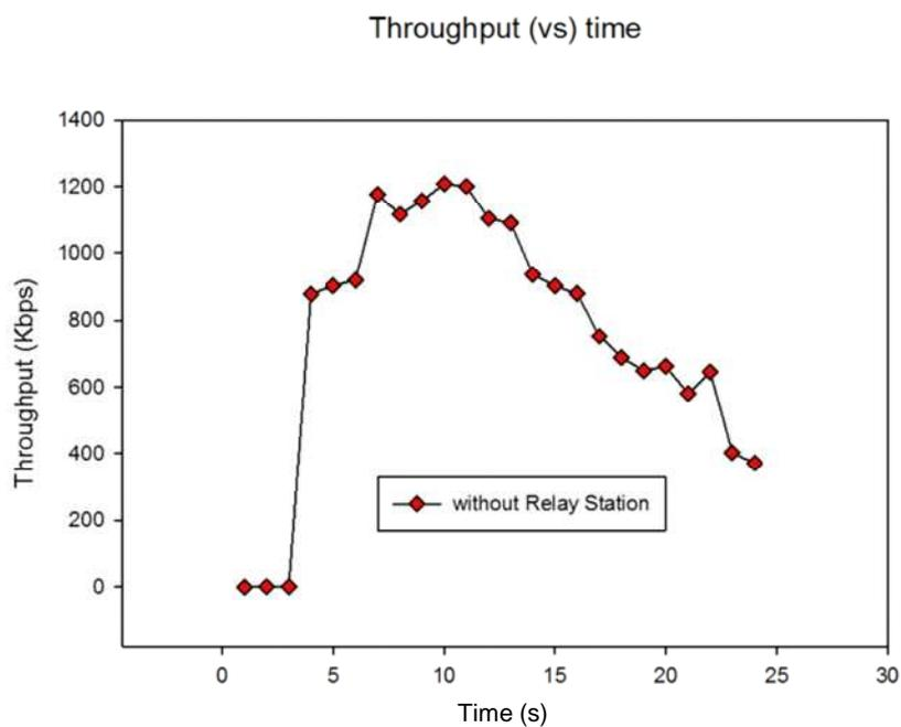
Figure 13. Throughput without relay station.
