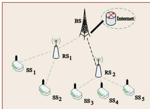
**Figure 1.** IEEE 802.16j mobile multi hop relay (MMR) network.
