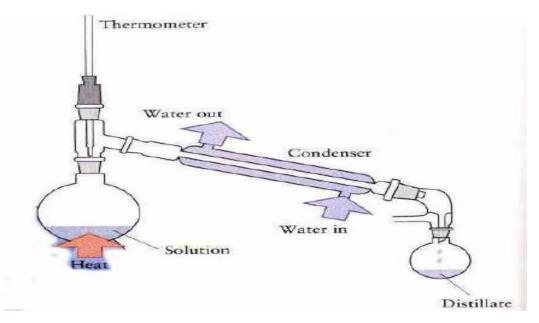
Figure 1. Schematic laboratory distillation equipment.
