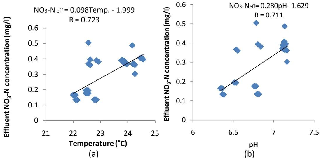
Figure 9. Graph of effluent NO<sub>3</sub>-N concentration vs (a) Temperature and (b) pH.
