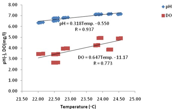
**Figure 5.** Variation of effluent pH and DO with temperature.
