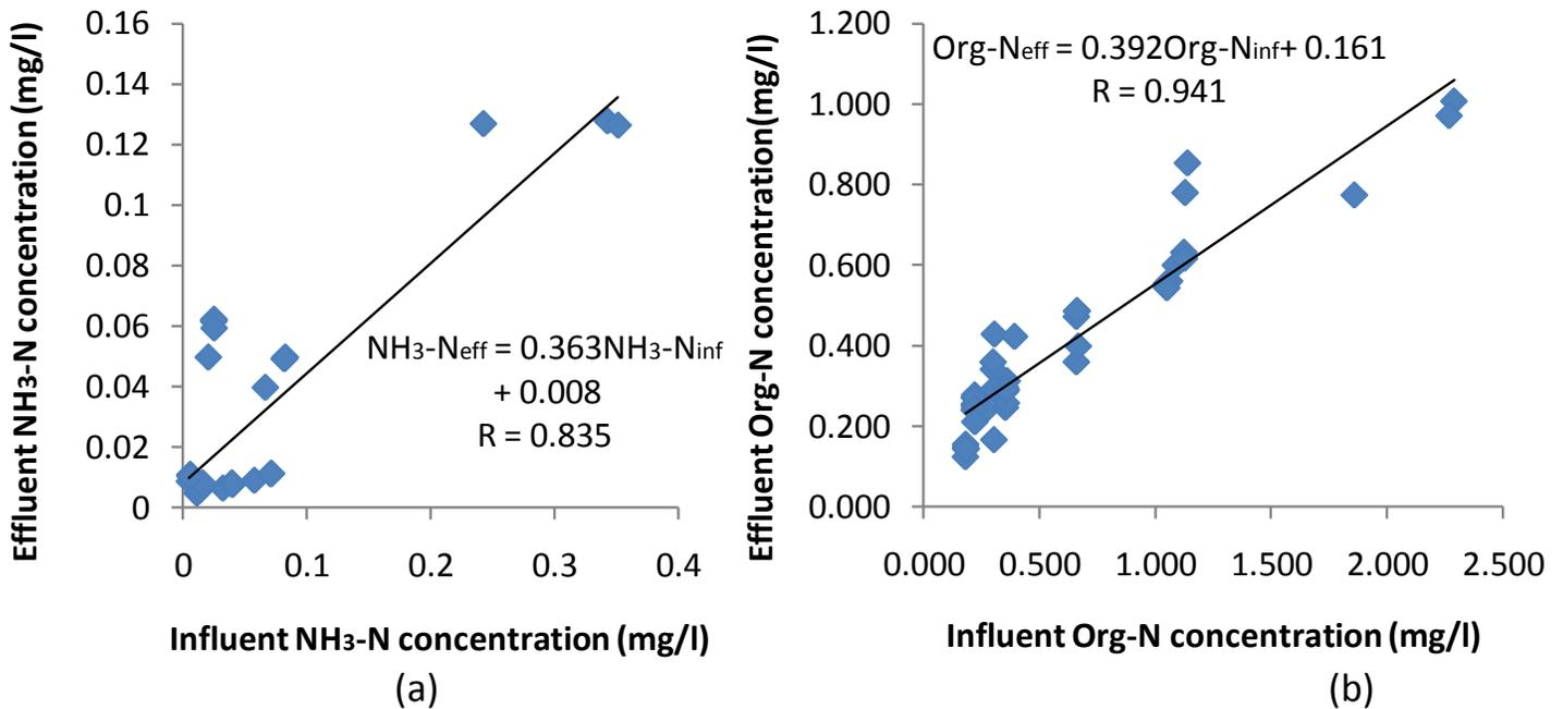
**Figure 7.** Variation of (a) Influent NH<sub>3</sub>-N and Effluent NH<sub>3</sub>-N and (b) Influent Organic Nitrogen and Effluent Organic Nitrogen.
