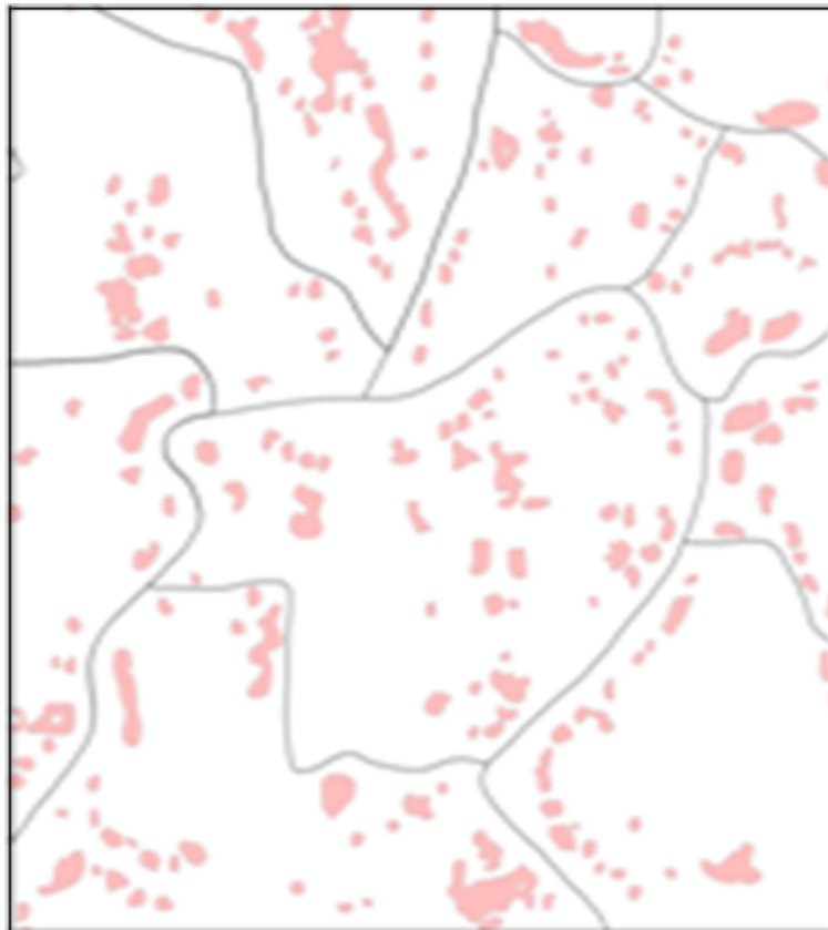
Figure 3. Settlements of a particular mauza differentiated by overlaying 'mauza' polygons and 'settlement' polygons
