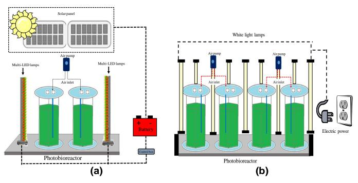
Figure 1. Types of lighting in farming systems. (a) Multi-LED lamps. (b) White light lamps.
