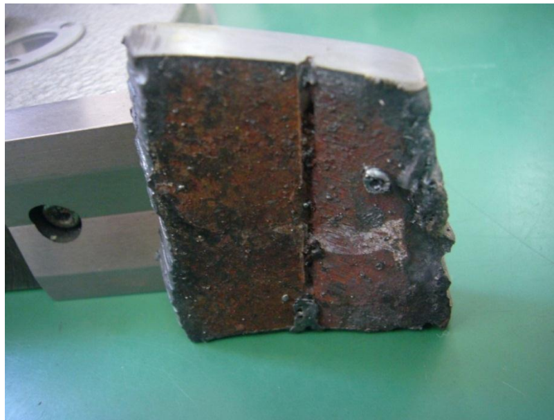
Figure 13. Discontinuity in weldment ( a = 2.5 mm; 2c = 100 mm).
