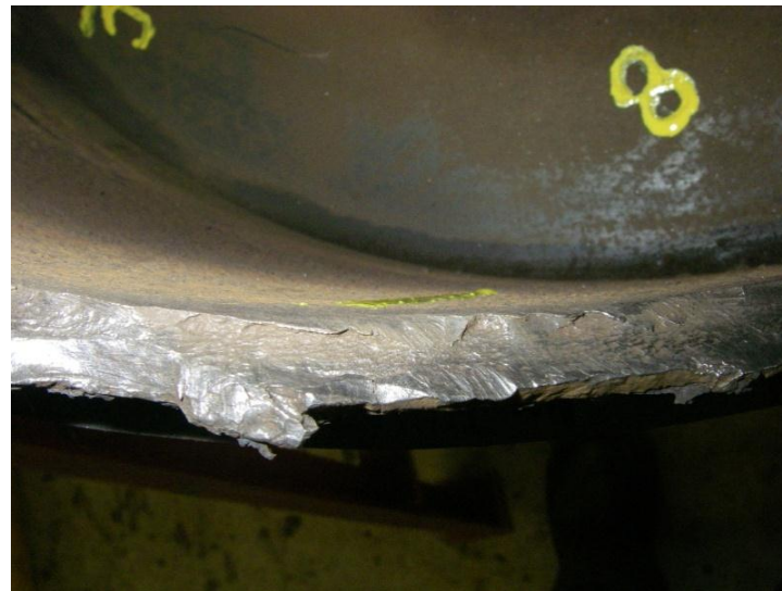
Figure 11. Zone of final fracture, point 8.
