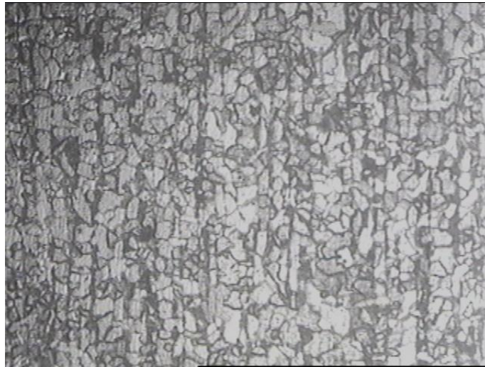
Figure 4. Disc-microstructure ferrite perlite [250X] (Hardness 135 HB) (Specification 119-159 HB).
