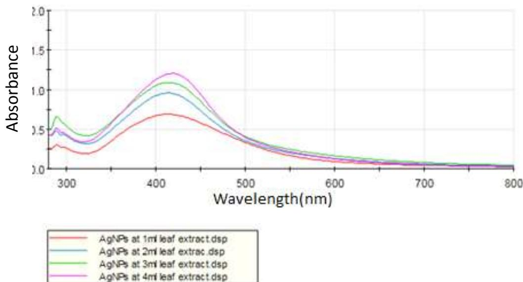
**Figure 5.** Absorption spectra of AgNPs of different amounts of *C. anguria* leaf extract (1, 2, 3 and 4 ml) with 10 of 1 M  $\text{AgNO}_3$  solution. The figure shows an increase of absorption intensity with an increase in the amount of leaf extract.
