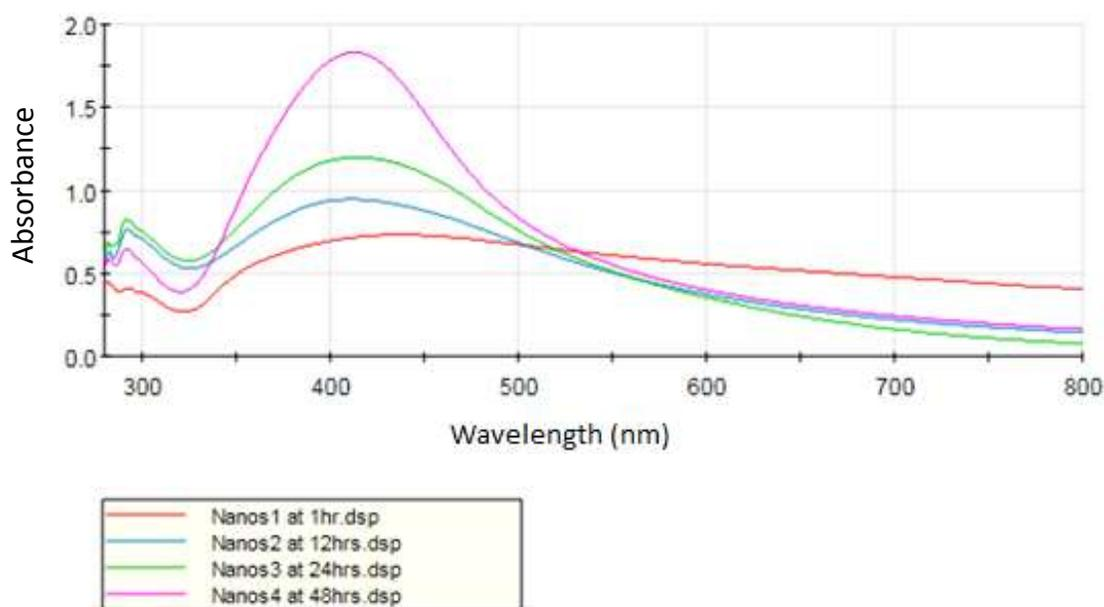
**Figure 3.** Absorption spectra of AgNPs (synthesized from 1 mM  $\text{AgNO}_3$  and *Cucumis anguria* leaf extract) observed at four different times. The figure shows an increase of absorption intensity as a function of reaction time.
