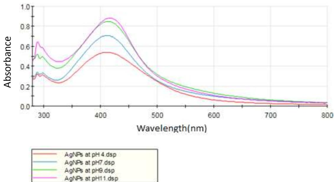
**Figure 4.** Absorption spectra of AgNPs (synthesized from 1 mM  $\text{AgNO}_3$  and *C. anguria* leaf extract) at different pH values (pH = 4, 7, 9 and 11).
