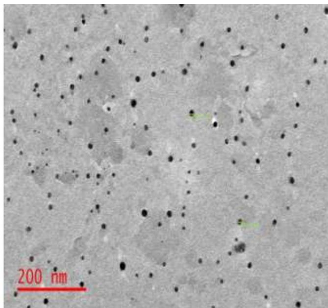
**Figure 8.** TEM images of silver nanoparticles at pH 7 scanned at 200 nm.
