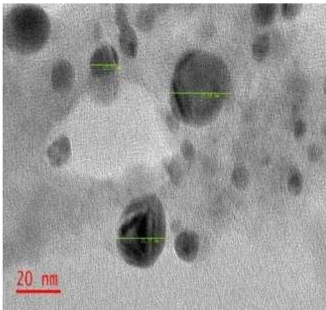
**Figure 7.** TEM images of silver nanoparticles at pH 4 scanned at 20 nm.
