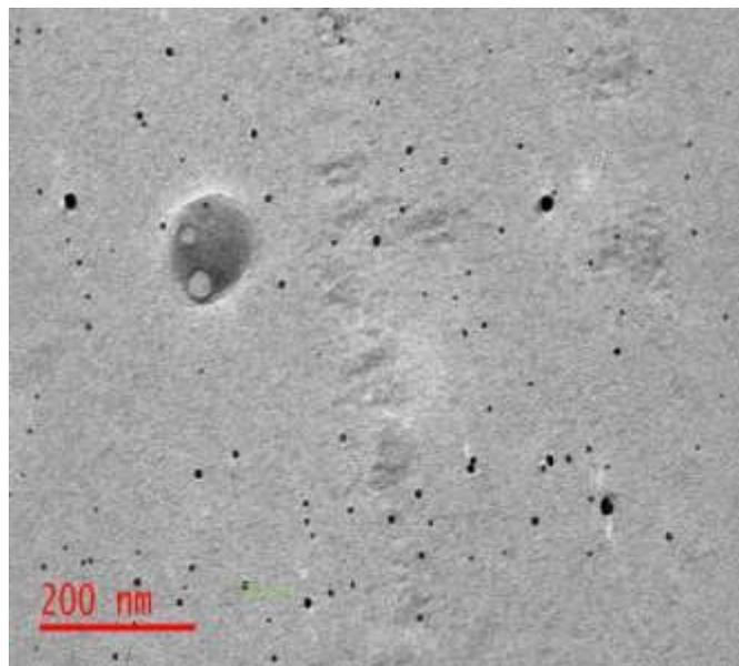
**Figure 9.** TEM images of silver nanoparticles at pH 11 scanned at 200 nm.
