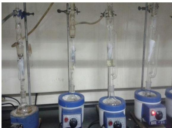
Figure 6. Soxhlet extraction experiment for the residues.
