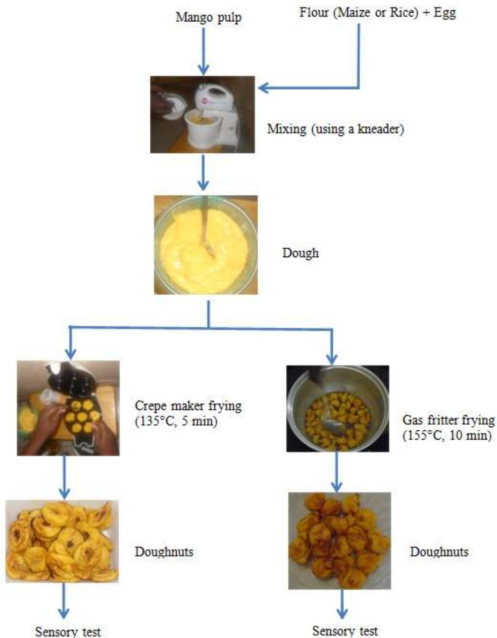
**Figure 1.** Diagram of mango doughnuts processing.
