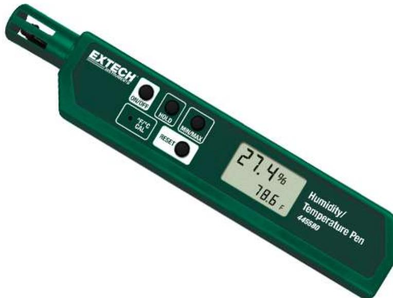
**Figure 6.** Extech 445580 Compact Digital Hygro-Thermometer pen.
