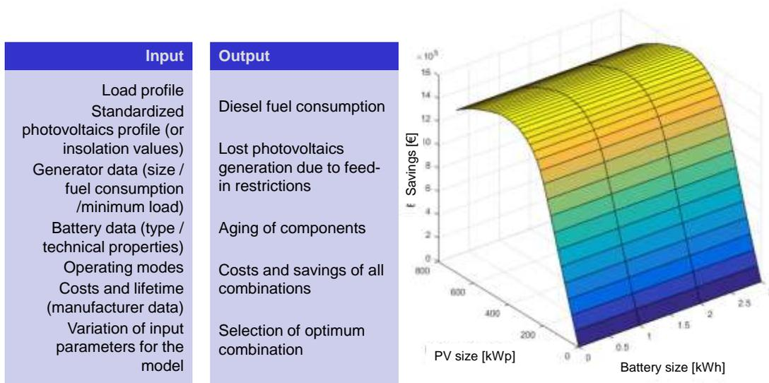
**Figure 5.** Input and output of modelling tool and results from specific analysis.
