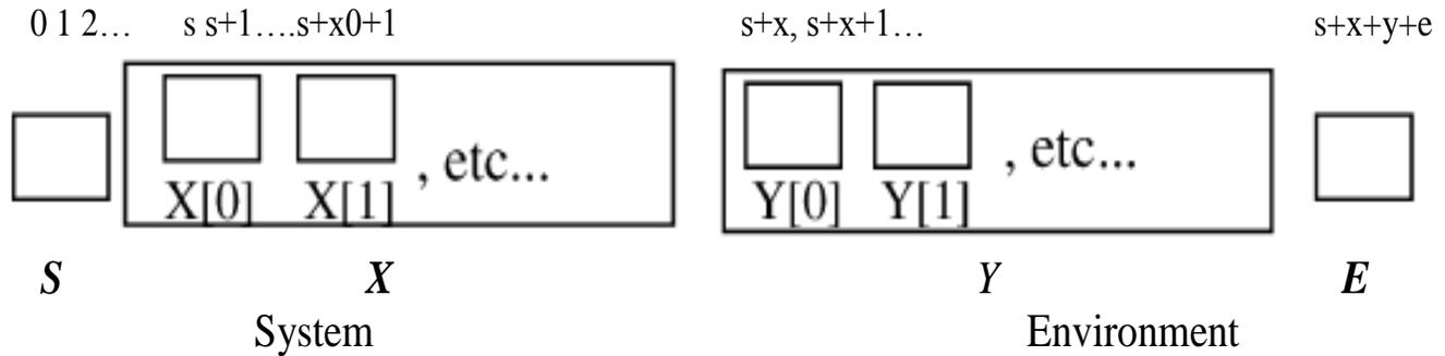
**Figure 1.** DMRG procedure and blocks labelling. To form the system, the blocks from vector of blocks  $X$  are added one at a time to block  $S$  while blocks from vector of blocks  $Y$  are added one at a time to  $E$  to form the environment. Blocks are vectors of integers. The numbers at the top of the figure, label all sites in a fixed and unique way (Alvarez 2009).
