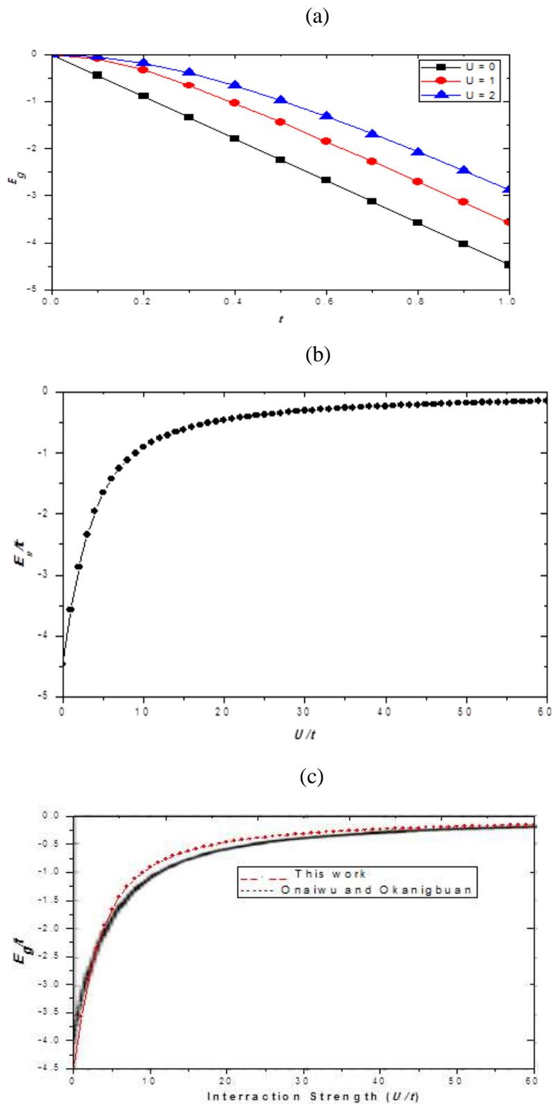
**Figure 2.** The plot of dispersion curve for four electrons on four sites (a) is the energy ( $E_g$ ) versus hopping energy ( $t$ ) at different values of Coulomb interaction ( $U$ ) as shown in the legend (b) Variation of  $E_g/t$  with the on-site energy  $U/t$  (c) shows similar result obtained from exact solution by Onaiwu and Okanigbuan (2013).
