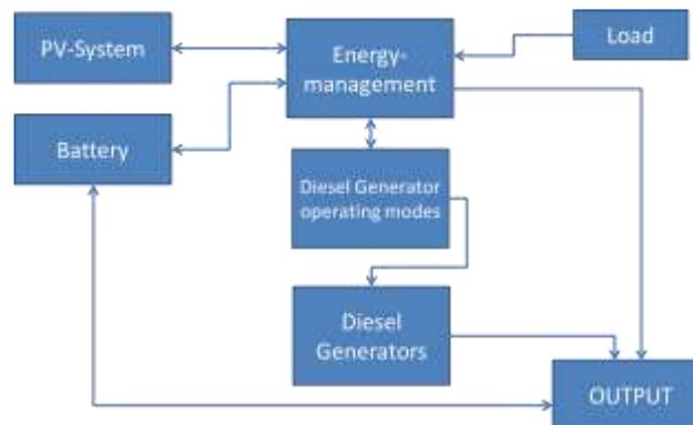
**Figure 4.** Setup of PV hybrid modelling tool .
