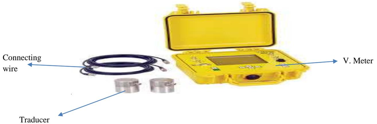
Figure 1. Ultrasonic pulse velocity.
