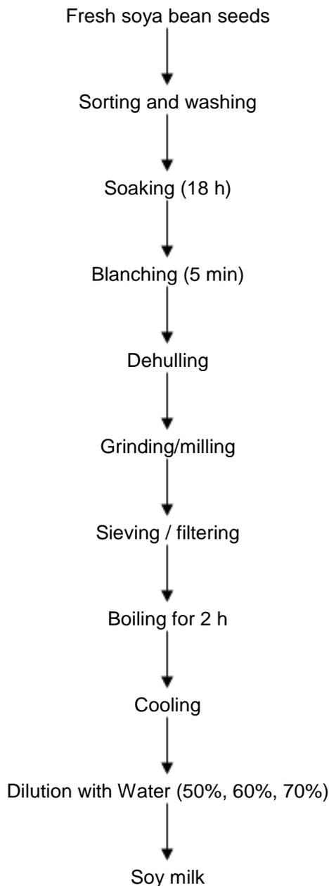
**Figure 4.** The flow chart for soymilk production.
