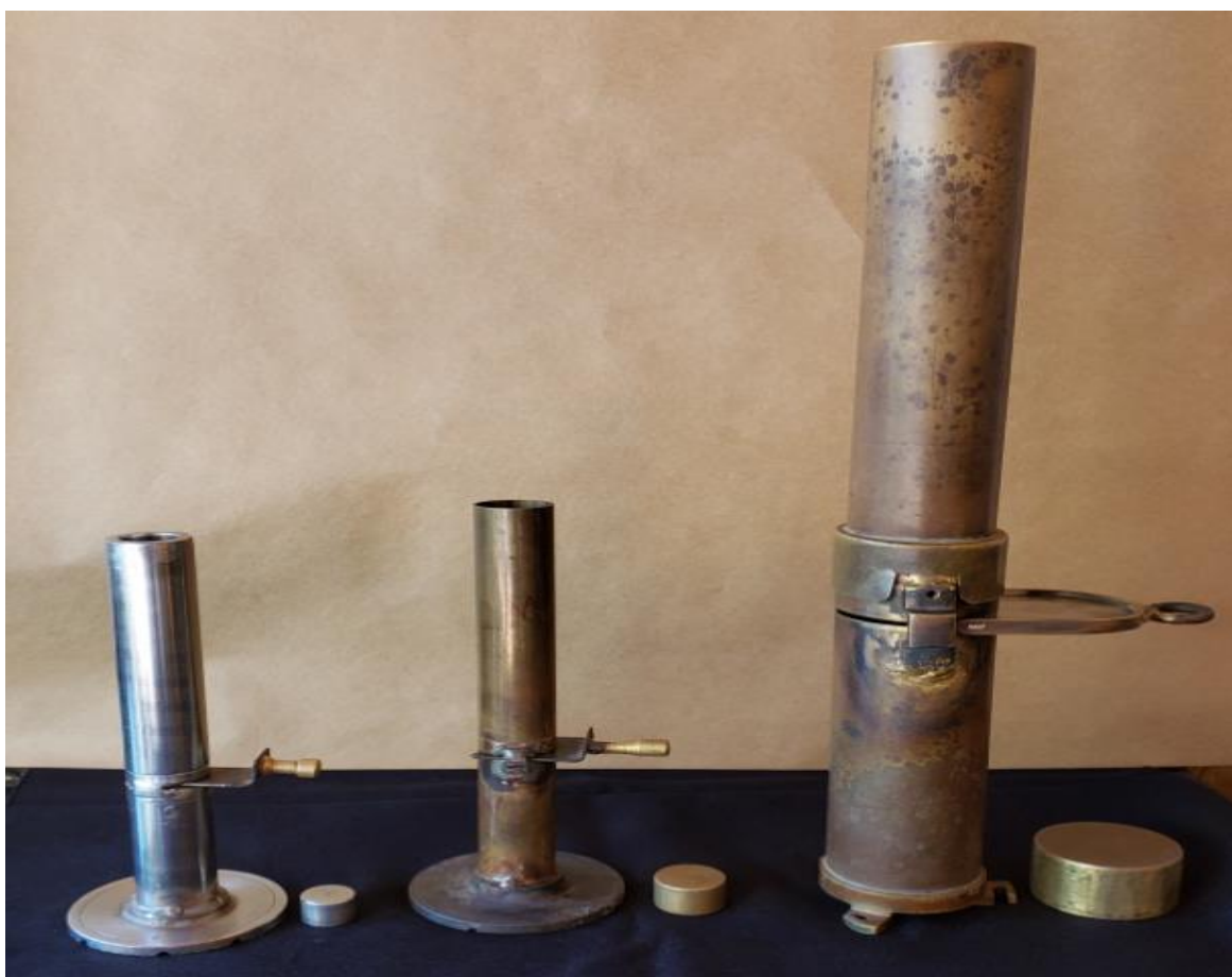
Figure 1. From left to right, the 15.30 ml and the 31.26 microchondrometers and the 250 ml chondrometer, with its respective pistons and cutter bars.
