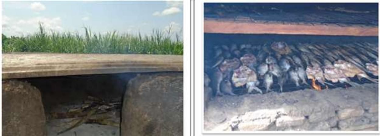
**Figure 2.** The structures of Pit (left) and *Chorkor* (right) smoking ovens.
