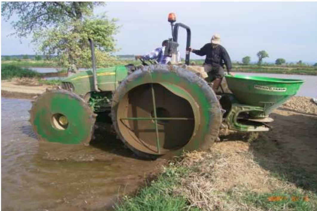
**Figure 1.** Paddy drilling with steel wheel tractor.
