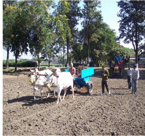
Figure 4. In field recording of pull and speed of operation with and without rotation of manure spreading auger
