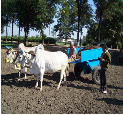
Figure 4. In field recording of pull and speed of operation with and without rotation of manure spreading auger
