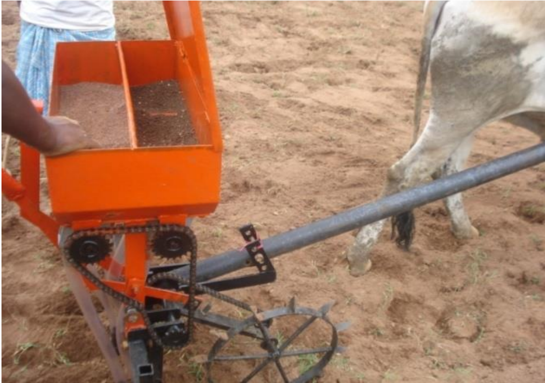
Figure 8. Bullock drawn seed cum fertilizer drill.
