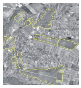
**Figure 3.** Importing and assessment of old sketches and maps into GIS, map of plots can be represented in a satellite image after geo-referencing.
