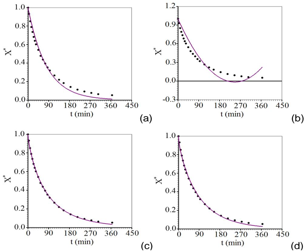
**Figure 2.** Drying kinetics at 50°C simulated by the model: (a) Lewis; (b) Wang and Singh; (c) Page; (d) Silva et al.
