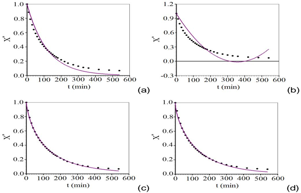
**Figure 1.** Drying kinetics at 40°C simulated by the model: (a) Lewis; (b) Wang and Singh; (c) Page; (d) Silva et al.
