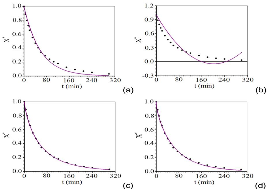
**Figure 3.** Drying kinetics at 60°C simulated by the model: (a) Lewis; (b) Wang and Singh; (c) Page; (d) Silva et al.
