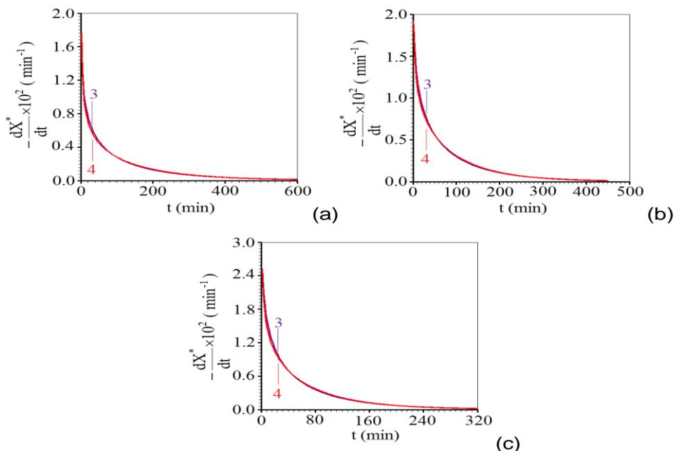
**Figure 4.** Drying rates calculated using the expressions obtained by the models 3 and 4 at temperature  $T =$ : (a) 40°C; (b) 50°C; (c) 60°C.
