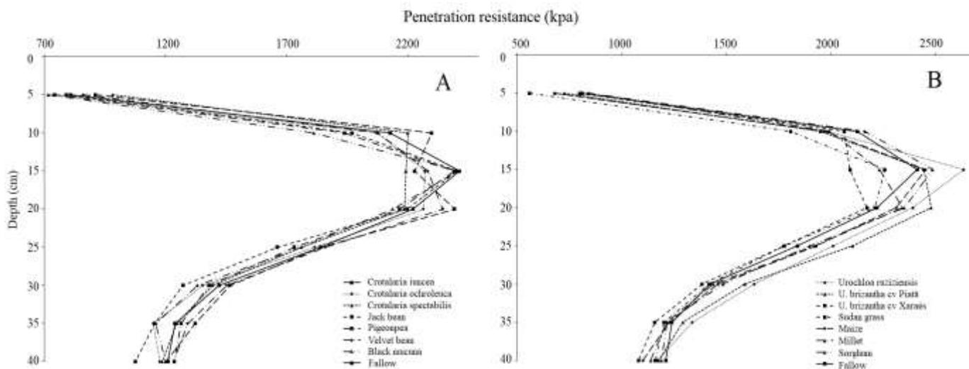
**Figure 2.** Average soil penetration resistance measurements over the 0 to 40 cm depth range for soils cultivated with legumes (A) or monocotyledonous plants (B).
