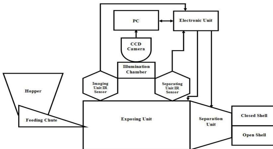
Figure 5. Block Diagram of the proposed system.
