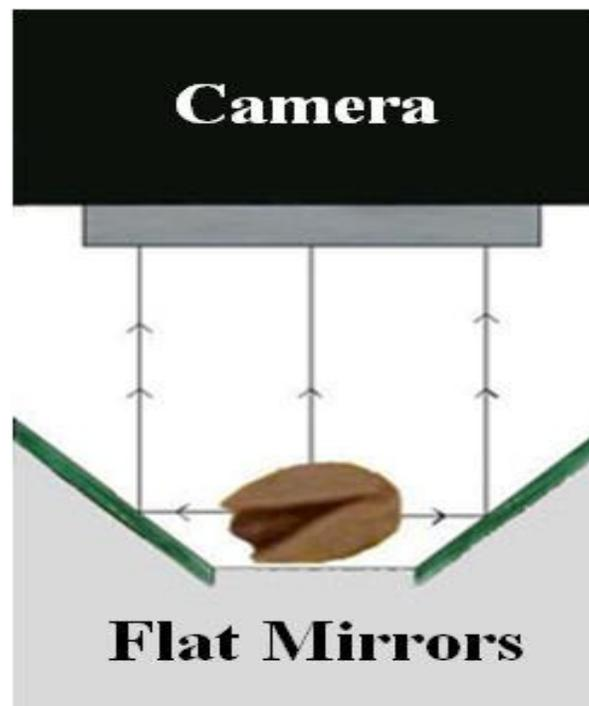
**Figure 3.** Arrangement of mirrors and camera.
