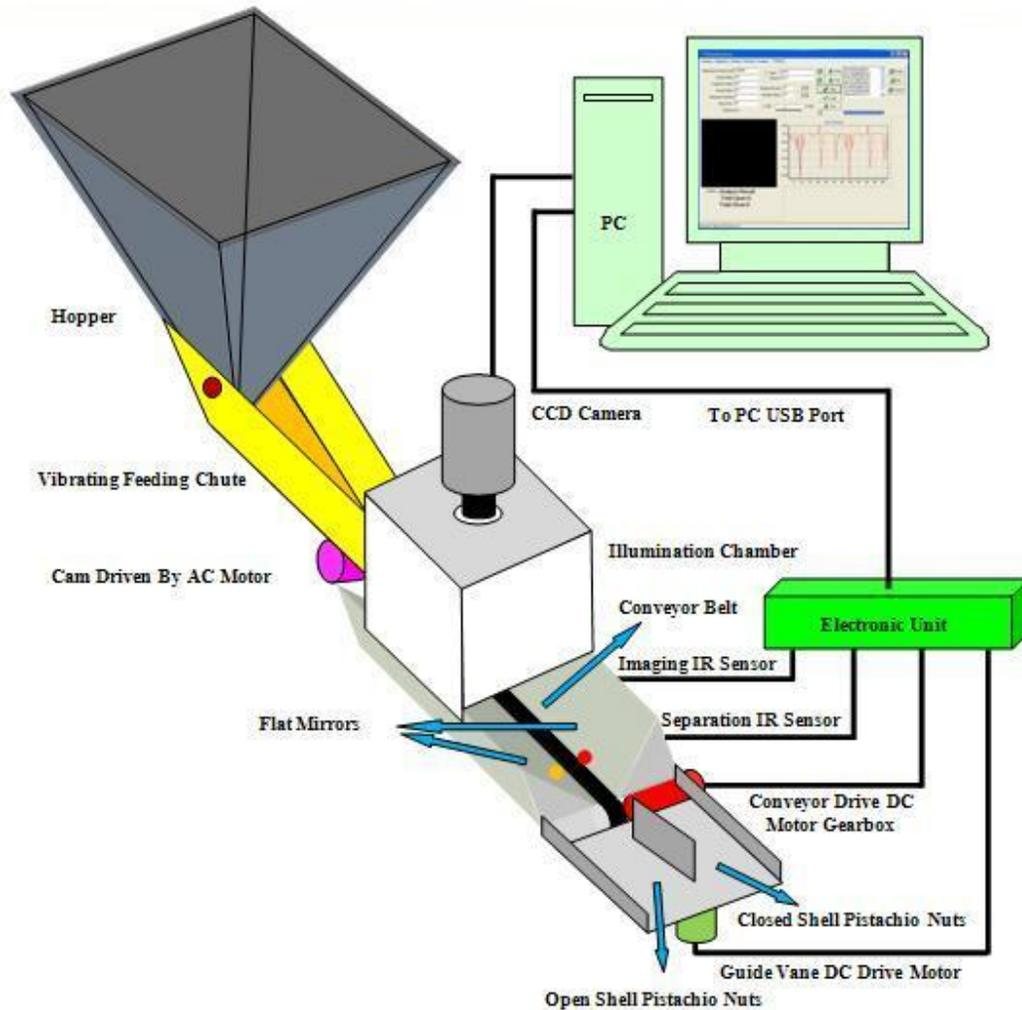
Figure 6. Schematic shape of sorting system.
