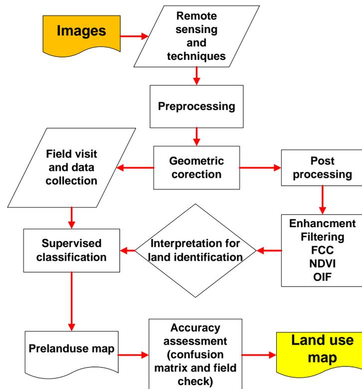
**Figure 2.** The general framework for image pre-processing, processing and post-processing.
