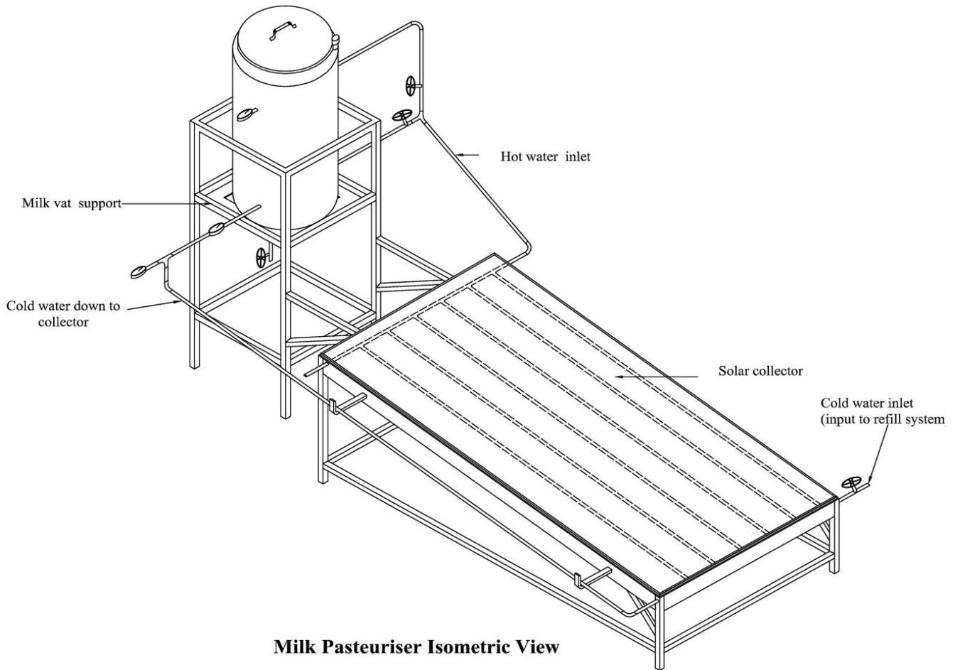
**Figure 2.** Isometric view of the solar milk pasteuriser showing the solar collector and milk container.
