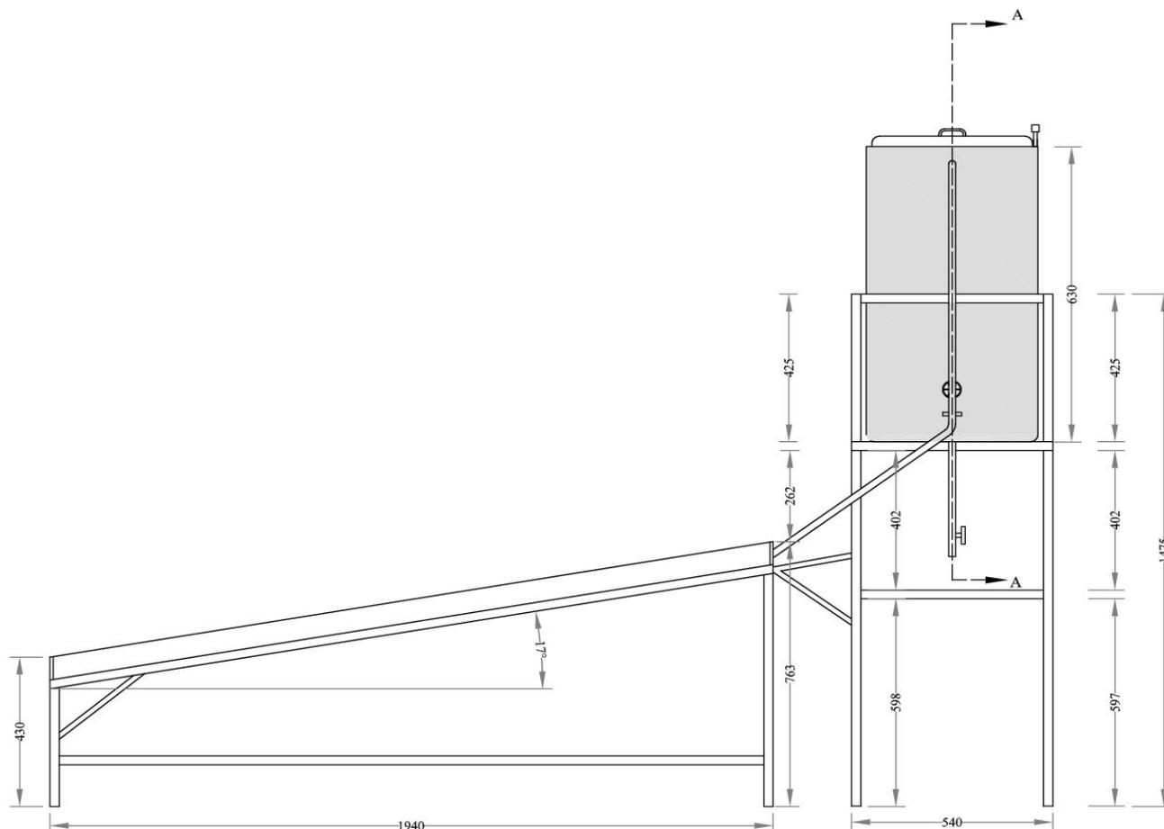
Figure 1. Side view of the solar milk pasteuriser (All figures in mm).
