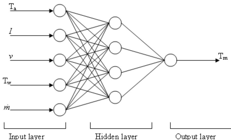
**Figure 3.** Structure of the ANN for the analysis of solar milk pasteuriser.  $T_a$ , Ambient air dry bulb temperature ( $^{\circ}\text{C}$ );  $I$ , solar radiation ( $\text{W}\cdot\text{m}^{-2}$ );  $v$ , wind speed, ( $\text{m}\cdot\text{s}^{-1}$ );  $T_w$ , temperature of hot water ( $^{\circ}\text{C}$ );  $\dot{m}$ , water flow rate through the collector ( $\text{kg}\cdot\text{s}^{-1}$ );  $T_m$ , temperature of milk ( $^{\circ}\text{C}$ ).
