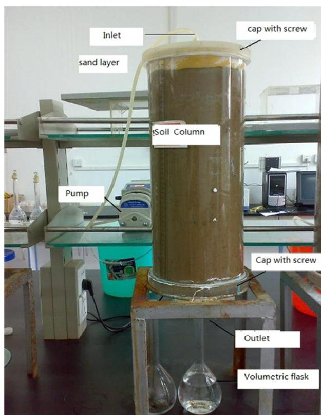
**Figure 1.** Experiment setup.
